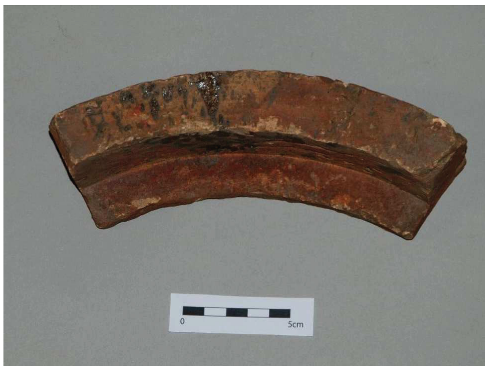
Plate 22: Sectional ring-sagger, No 1
