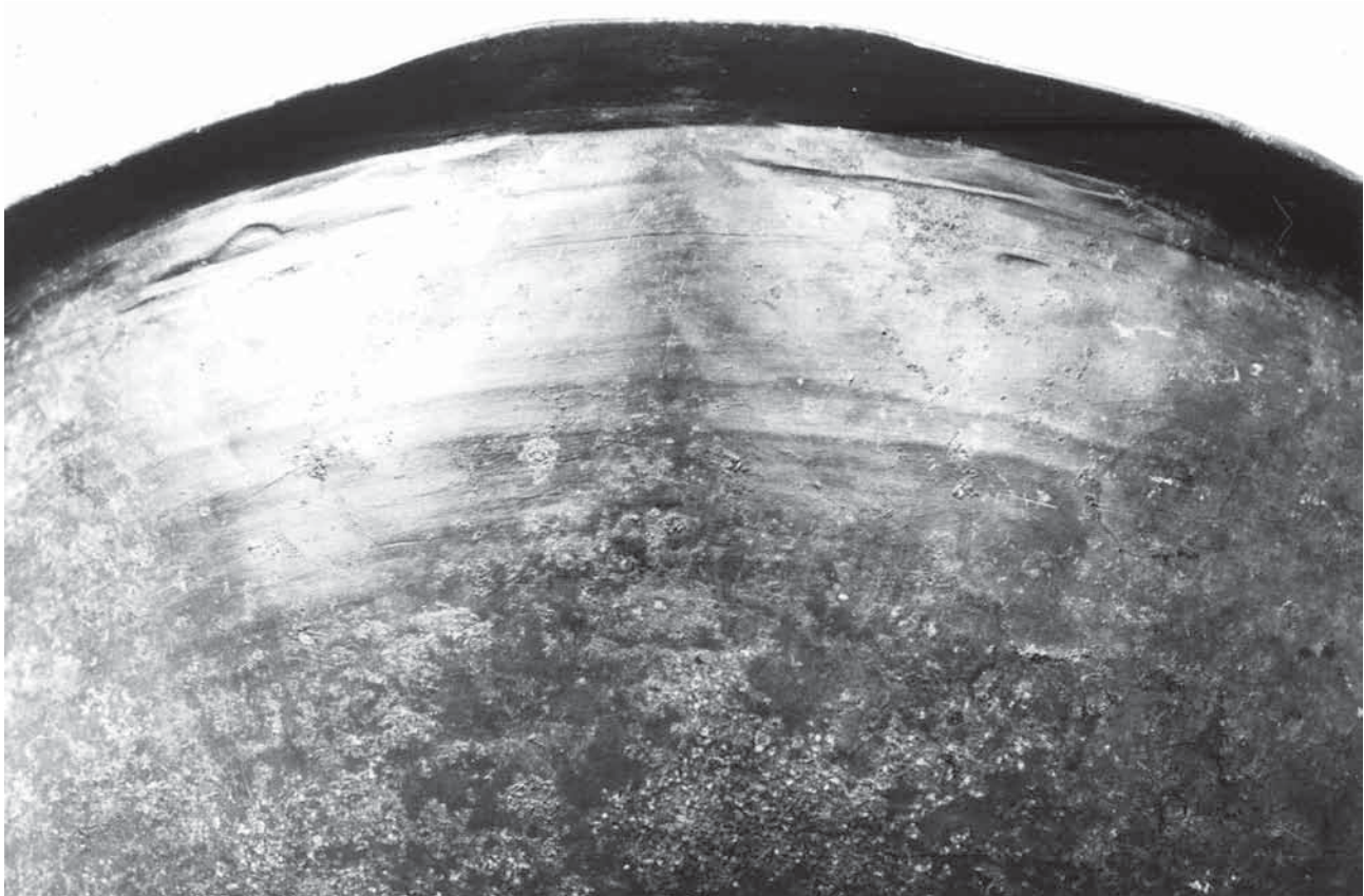
Fig.1397 Detail of copper alloy bowl 15150 showing turning marks
