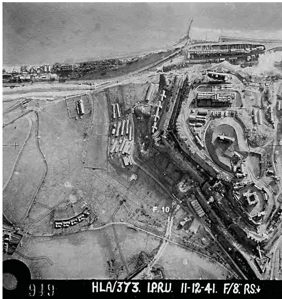
Plate VII , Aerial photograph dated 1941 showing line of anti-tank ditch (F. 10) running between Horseshoe Bastion and the East Wing Battery of Fort Burgoyne (image provided by Dover Museum)
