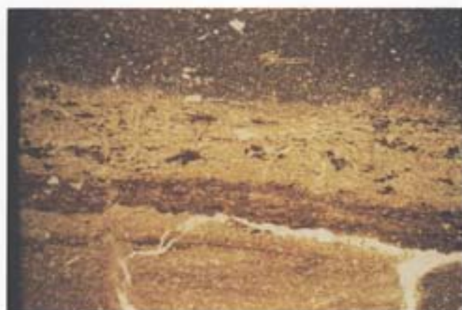
Fig 83g GTP 25: sample 27; projected microfiche reader view of Units 4c, 5a, and 5b. Bottom; mainly massive Unit 4c becoming weakly laminated at the top. Centre; dark brown Unit 5a with a basal laminated organic layer succeeded by a more mineralogenic layer containing organic fragments. Top; massive grey Unit 5b marl containing crushed and flattened mollusc fragments (upper centre right of photo). Frame length 0.11mm
