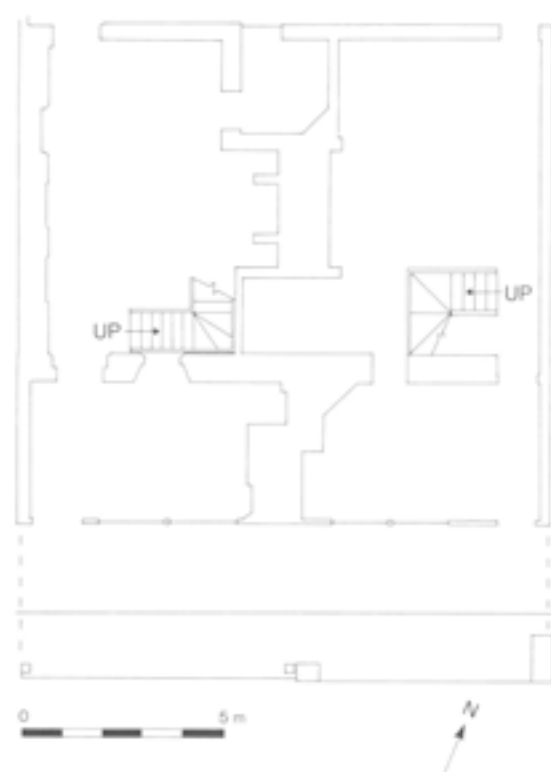
Fig 84 Row-level plan of 38–42 Watergate Street showing chimney stack and staircases inserted into the medieval hall
