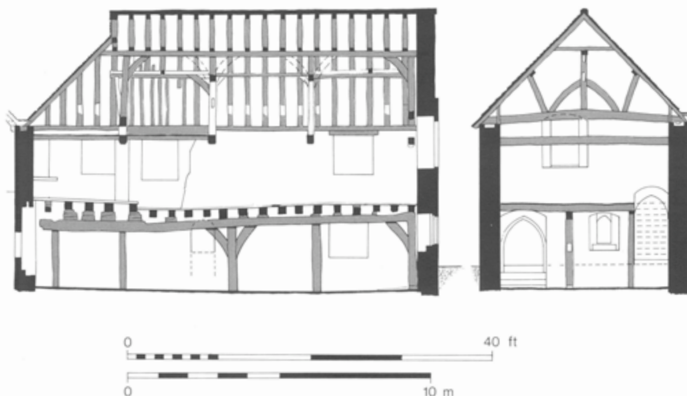
Fig 53 Cross section of the Marlipins, Shoreham, showing the timber arcade (after Packham 1924)
