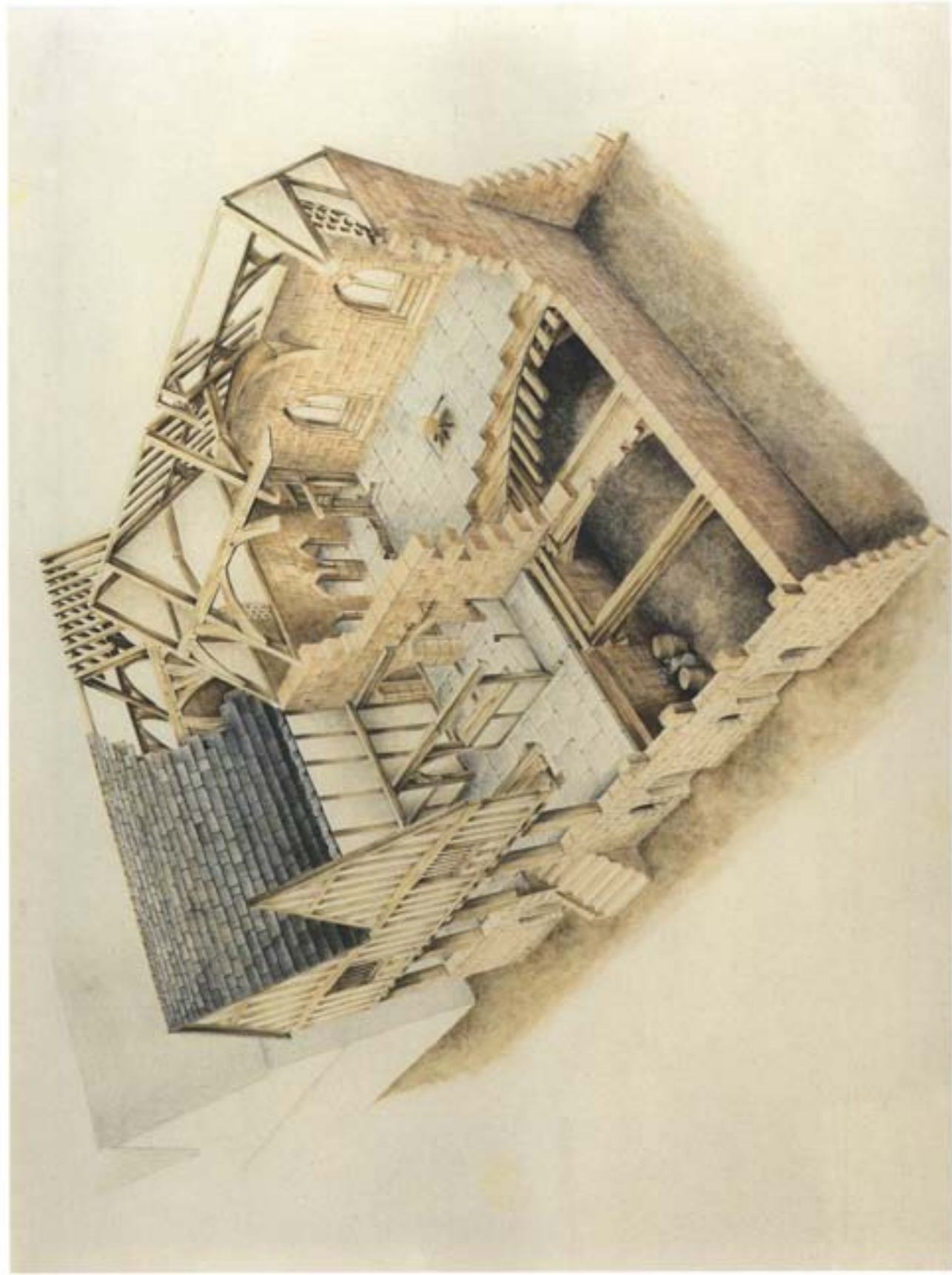
Plate 1 Cutaway reconstruction of medieval form of 38-42 Watergate Street (Graham Holmes)
