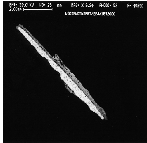
ILLUS 18b SEM-BS image of WE18.2 showing steel 'insert' within low carbon envelope (WE18.1): layer of iron oxide surrounds remaining metal core (bar = 2 mm)
