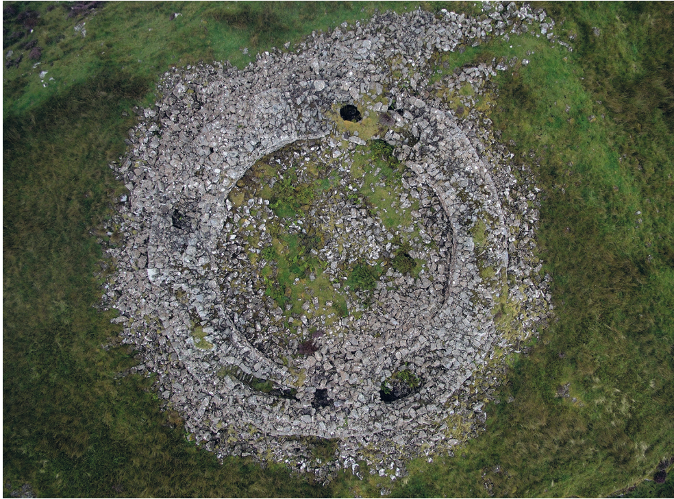
ILLUS 4 Low altitude vertical and oblique aerial photography uses a remote controlled microcopter equipped with a digital camera. This rectified vertical image captures the structural plan of Dun Suladale on Skye (NG 374 525)
