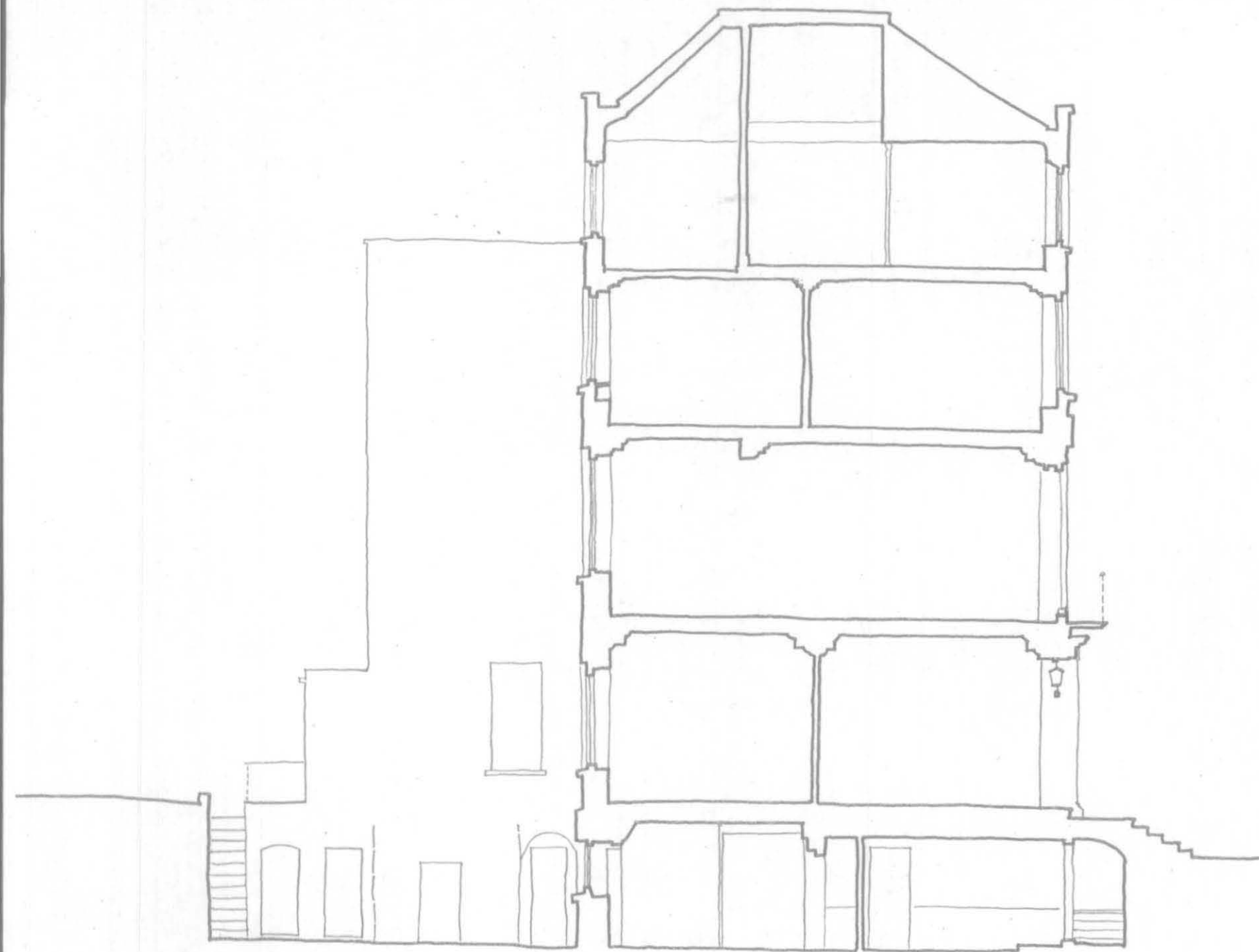
Fig 13 Sectional elevation from north to south through centre of building, looking east (1:100)
