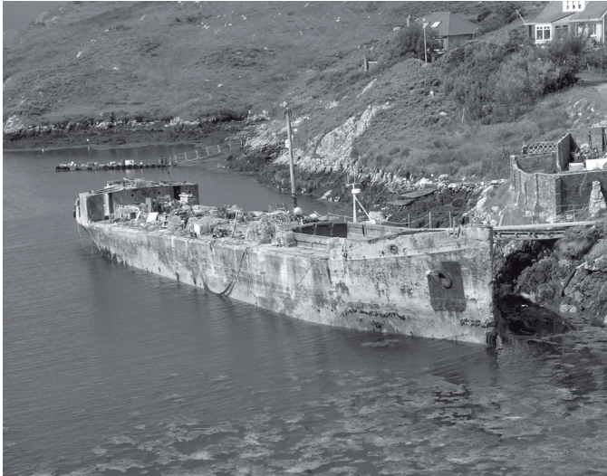
Few concrete boats survive, but this one, the 'Cretetree' is still used for storage and working purposes in the N harbour on Scalpay.
