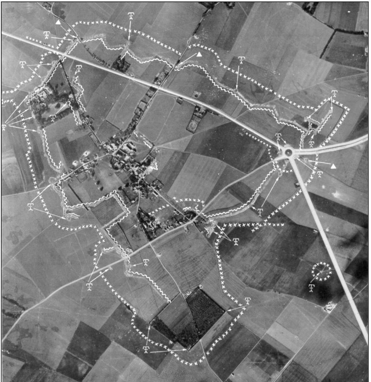
Fig. 4 - A Luftwaffe air photograph [undated, but probably taken in August 1940] showing the defences of St. Nicholas at Wade, just over a mile to the north of Sarre. The extensive perimeter defences of barbed wire [small crosses] and slit trenches [sinuous lines] were probably replicated at Sarre.
