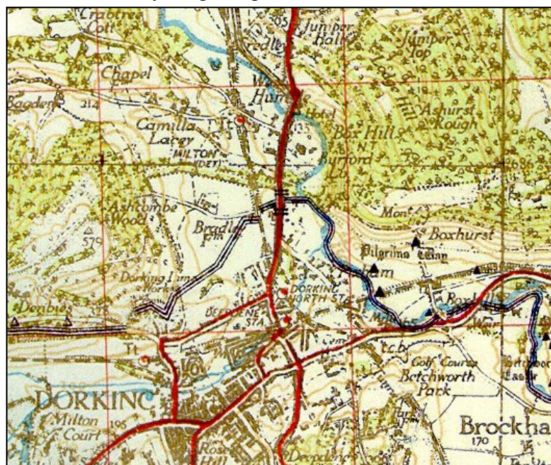
Fig. 2 - Portion of a German map (using an Ordnance Survey base) overprinted with defence works plotted from aerial reconnaissance. The line of the machine-dug anti-tank ditch to the west of the A24 road can be seen. To the east, the River Mole formed the principal anti-tank obstacle. 3
