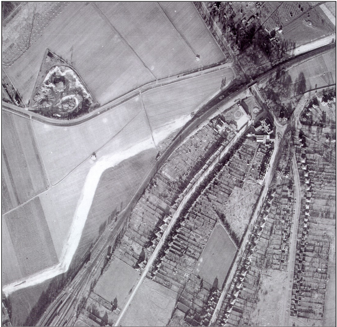
Fig. 3 - The filled in line of the anti-tank ditch, with pillboxes alongside it, shows very clearly in this RAF aerial photograph taken in January 1946. To the east of the Drift Bridge, the line is continued by anti-tank cubes in the woodland, and then by a further section of ditch.
