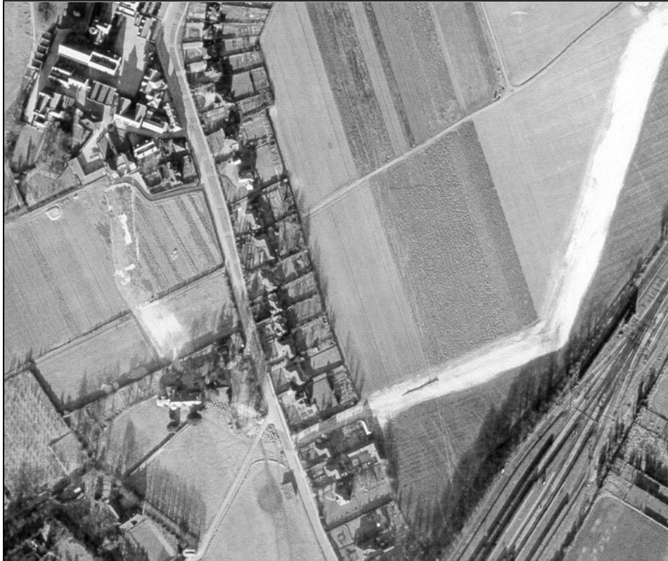
Fig. 4 - An air photograph taken in January 1946 shows the line of the infilled anti-tank ditch turning north after crossing Lansdown Lane South, and continuing through a forest of anti-tank cubes to the buildings of Epsom College
