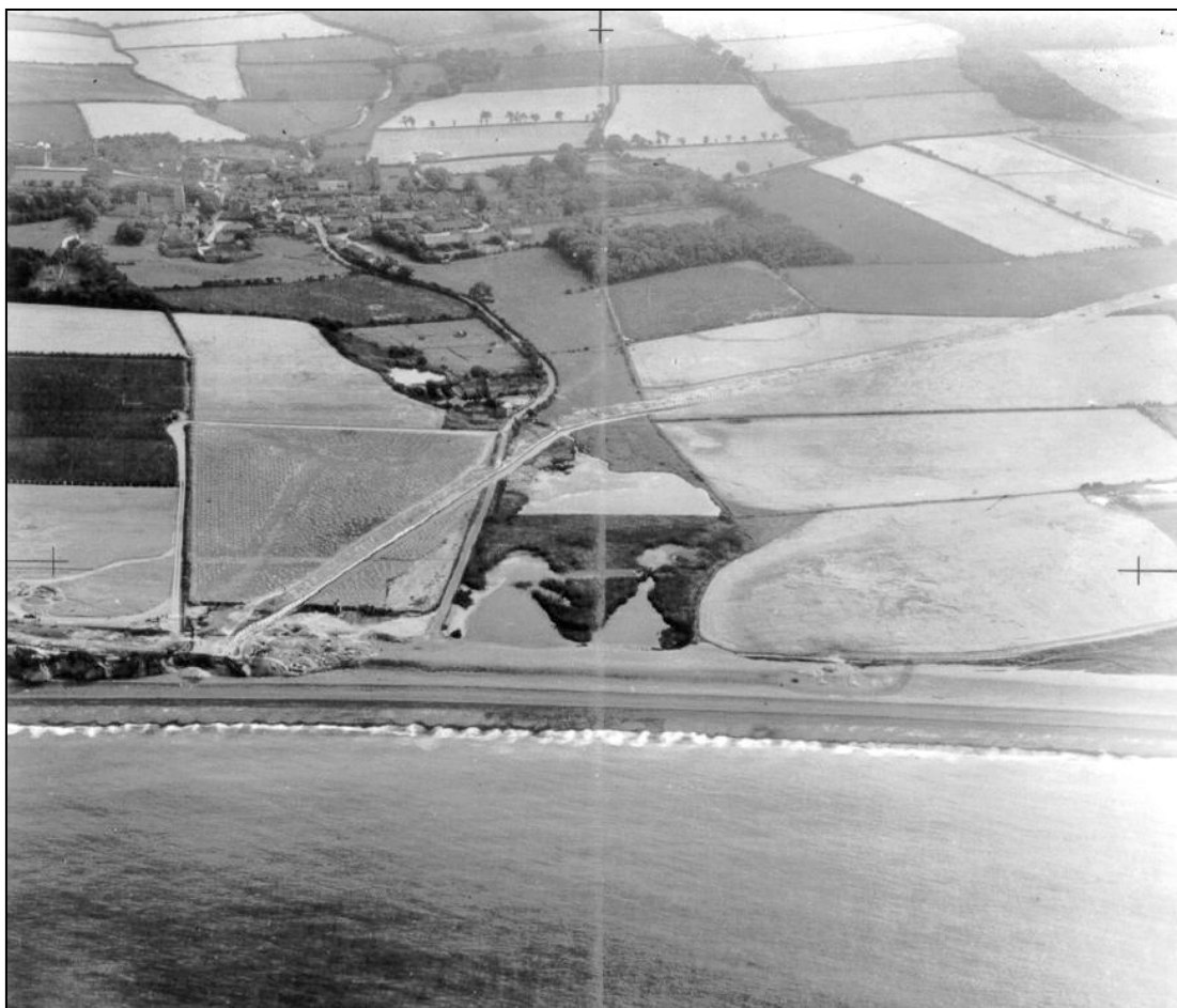
Fig. 7 - RAF oblique aerial photograph taken in August 1940, showing the revetted anti-tank ditch ending at the Weybourne Hope beach. This point was very heavily defended, and some of the defence works can be seen in the photograph.
