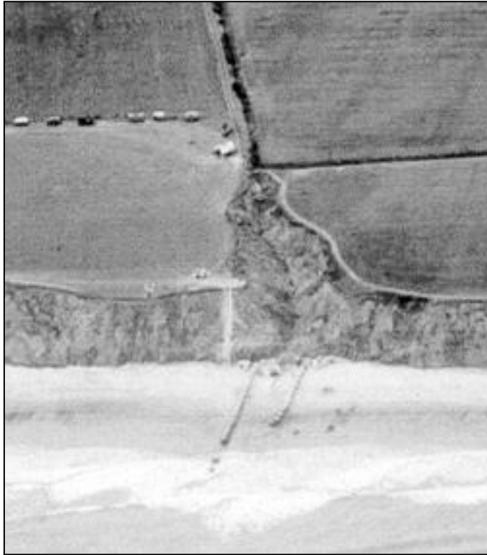
Fig. 11 - Parallel lines of anti-tank cubes running towards the sea at Atwick Gap can be seen in this detail from an oblique air photograph of July 1940. They were designed to prevent enemy armoured vehicles from traversing the beach to gain access to this exit through the cliffs.
