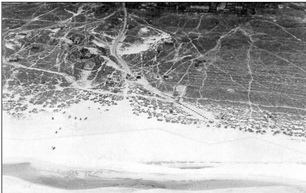
Fig. 7 - Aerial photograph taken on 16 August 1940, showing the first line of anti-tank blocks to be built. A pillbox is at the end nearest the sea, and a zig-zag line of barbed wire runs at the head of the beach. Behind, various structures can be seen within the sand dunes.
