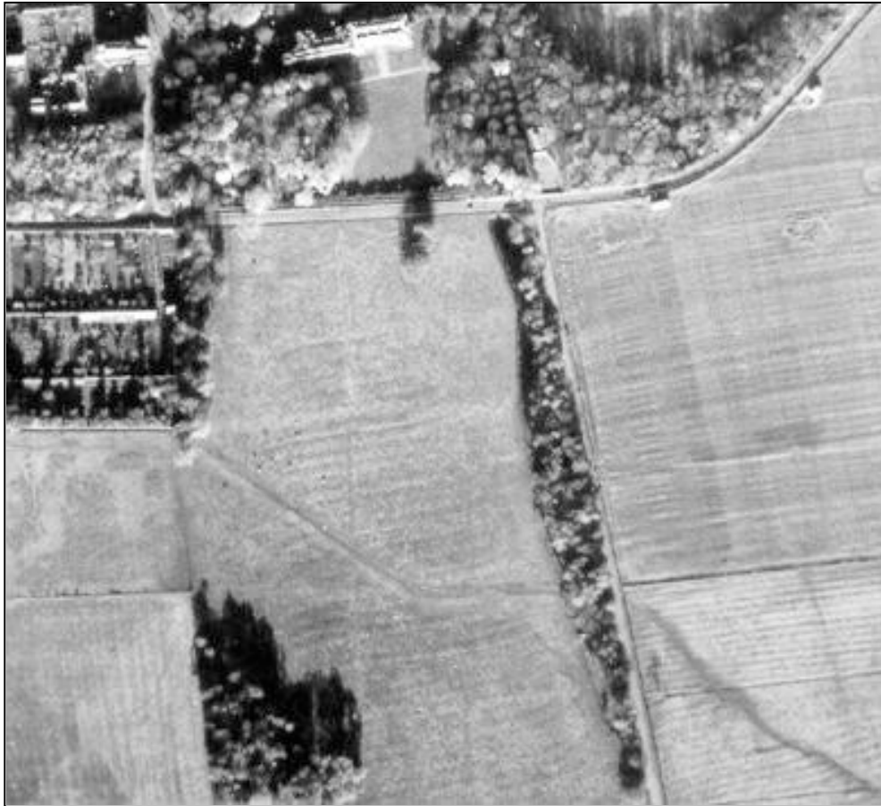
Fig. 4 - Detail from a November 1946 air photograph showing the course of the anti-tank ditch running from Turners Hospital at the south of Kirkleatham. To the west of the road (Fishponds Road) it has been filled in, but to the east it is still open.
