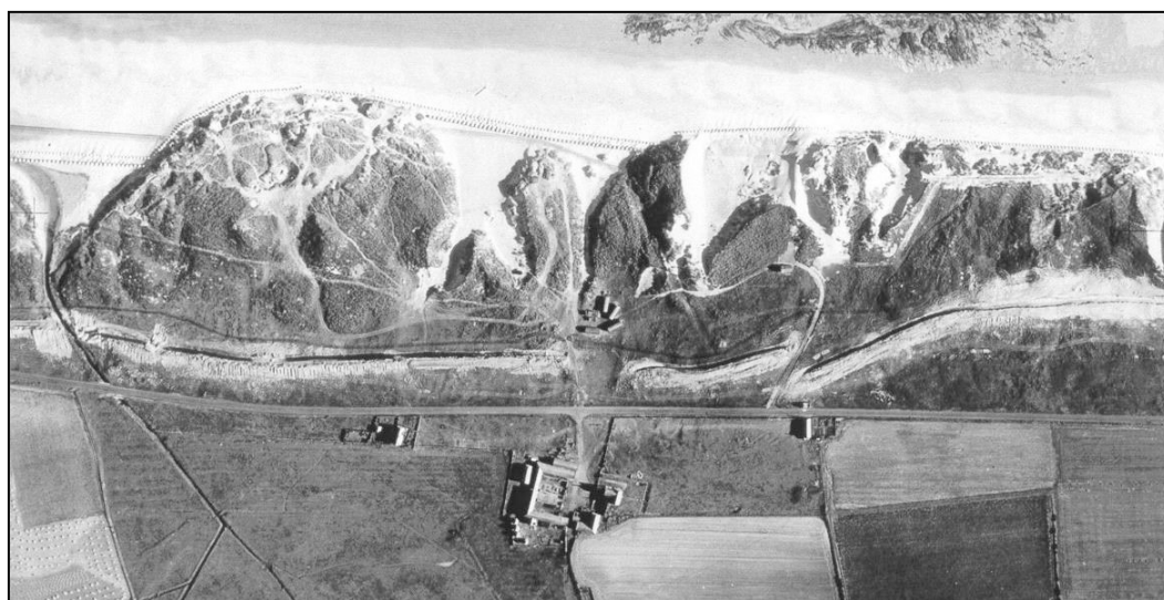
Fig. 3 - Beach front defences at Hemscott in a 1941 air photograph. The anti-tank ditch running between the road and the sand dunes can be seen, as can lines of anti-tank cubes and scaffolding blocking beach exits. The coast battery is positioned amongst the sand dunes: its accommodation huts are clearly visible, and it is possible to make out the gun positions.
