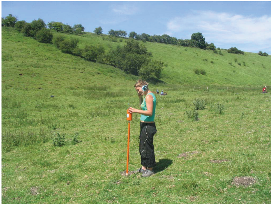
Figure 132 The use of a metal detector before augering
