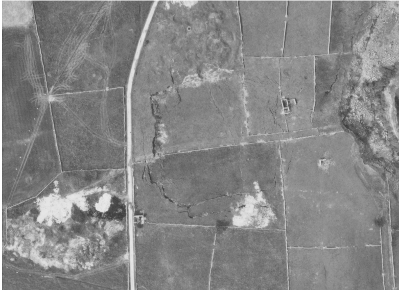
Figure 33. Subsidence caused by subterranean mining activity, Middleton. NMR MAL/75048 67 15-JUL-1975 © Reserved
