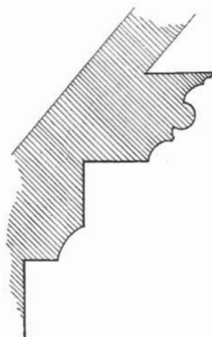
FIG. 12. SECTION OF FIFTEENTH-CENTURY ROOF-PLATE 47, HIGH STREET, AMERSHAM
