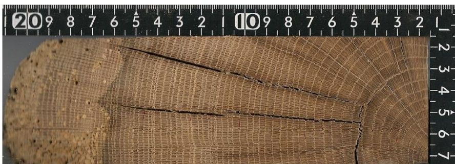
Photo 4: Section of oak from the east end of Beam 6 (series INMI01A)
