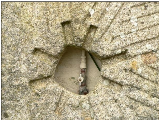
Millstone 6: detail of eye and rynd chases
