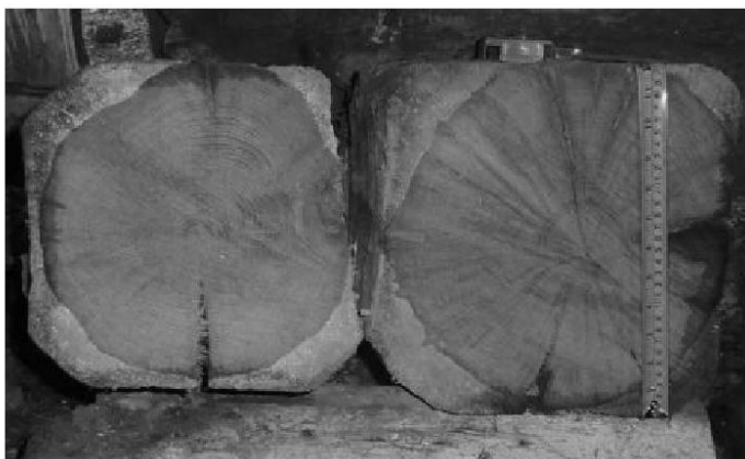
Photo 3: Two sections of oak sawn from Beam 6
