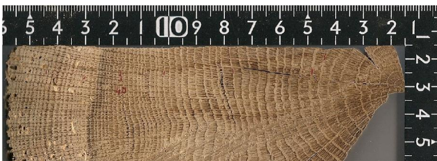
Photo 5: Section of oak from the west end of Beam 6 (series INMI01B)
