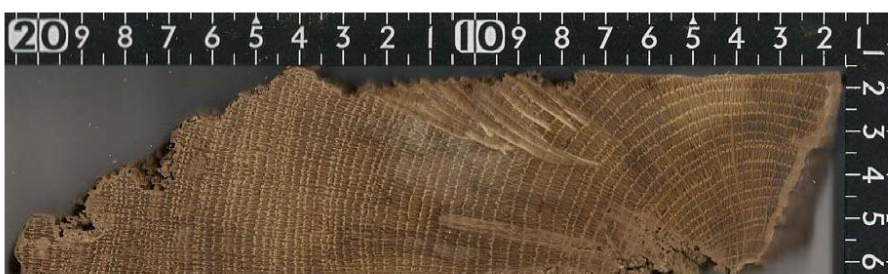
Photo 6: Section of oak from Joist 4 (series INMI02)
