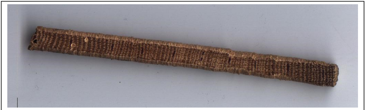
Core sample STH-F03 from the north-west purlin. Its 94 rings span the years 1393 - 1486
