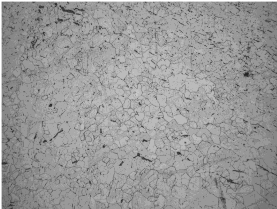
Figure Microstructure of comparative uniform sized grains but also local high density of small slag inclusions
