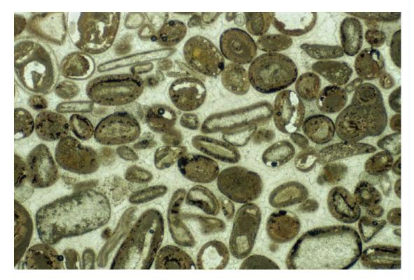
Sample: 4 SF: 833 Item: cornice / architrave Width of View of Picture: 3.4 mm Petrographic type: bioclastic oolitic grainstone with drusy spar cement Grain overcompaction: none Distinguishable bioclasts: miscellaneous calcite-replaced molluscs.
