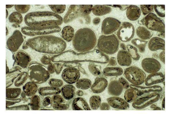
Sample: 16 SF: 697 Item: part of lathe-turned stub Width of View of Picture: 3.4 mm Petrographic type: bioclastic oolitic grainstone with drusy spar cement Grain overcompaction: moderate; some interpenetration, crushing of micrite envelopes, and spalling of superficial layers on ooliths. Areas of white space in some of the oolith cortices are due to fracture of the grains during the section-making process.
