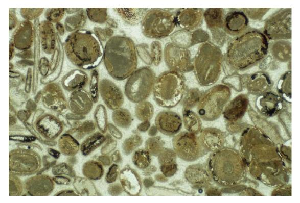
Sample: 3 SF: 664 Item: uncompleted sump Width of View of Picture: 3.4 mm Petrographic type: bioclastic oolitic grainstone with drusy spar cement Grain overcompaction: none Areas of white space in some of the oolith cortices are due to fracture of the grains during the section-making process. Distinguishable bioclasts: echinoderm; miscellaneous calcite-replaced molluscs; probable brachiopod.
