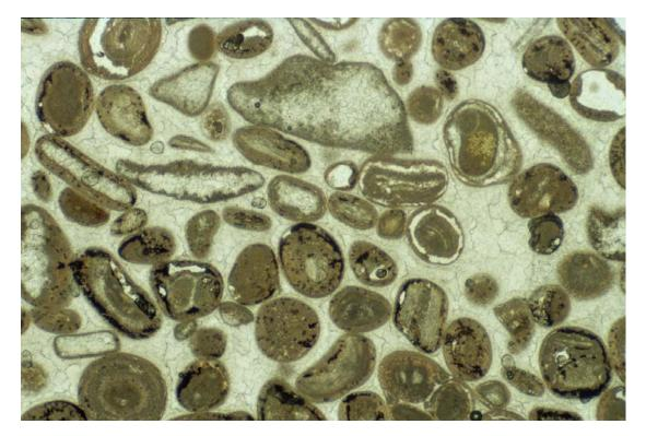
Sample: 17 SF: 358 Item: waster from coping stone Width of View of Picture: 3.4 mm Petrographic type: bioclastic oolitic grainstone with drusy spar cement Grain overcompaction: none Areas of white space in some of the oolith cortices are due to fracture of the grains during the section-making process. Distinguishable bioclasts: some calcite-replaced probable mollusc fragments
