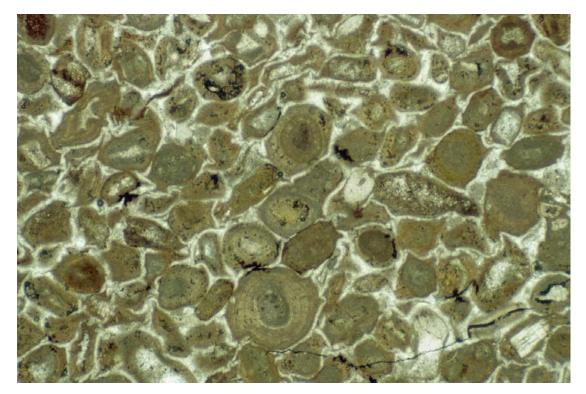
Sample: 11 SF: 855 Item: scappled block Width of View of Picture: 3.4 mm Petrographic type: oolitic grainstone with drusy spar cement Grain overcompaction: strongly overcompacted after 1<sup>st</sup> cement generation to produce fitted fabric and crushing of ooid cortices. Areas of white space in some of the oolith cortices are due to fracture of the grains during the section-making process.
