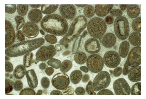
Sample: 9 SF: 750 Item: large box, post 1850 Width of View of Picture: 3.4 mm Petrographic type: bioclastic oolitic grainstone with drusy spar cement Grain overcompaction: none Distinguishable bioclasts: miscellaneous calcite-replaced molluscs as oolith nucleii; probable oyster forming oolith nucleus upper centre
