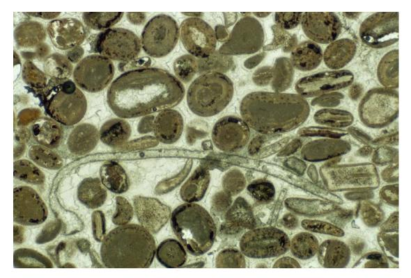
Sample: 7 SF: 597 Item: lip of candlebox Width of View of Picture: 3.4 mm Petrographic type: bioclastic oolitic grainstone with drusy spar cement Grain overcompaction: none Distinguishable bioclasts: echinoderms; miscellaneous calcite-replaced molluscs, including large example across middle of frame.
