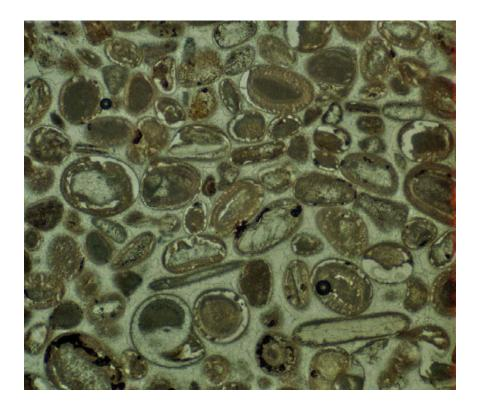
Sample: 1 SF: 718 Item: lathe-turned baluster Width of View of Picture: 2.8 mm Petrographic type: oolitic grainstone with drusy spar cement Grain overcompaction: none Areas of white space in some of the oolith cortices are due to fracture of the grains during the section-making process. Distinguishable bioclasts: micromorphic gastropod.
