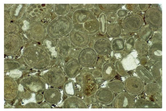
Sample: 18 SF: none Item: from core, 5 mm below hardground at top of Coombe Down Oolite Width of View of Picture: 3.4 mm Petrographic type: bioclastic oolitic grainstone with thin 1st generation isopachous calcite cement and vadose silt filling remaining intergranular pore space. Grain overcompaction: none Distinguishable bioclasts: broozeen forming colith nucleus ten left: achinederm with
