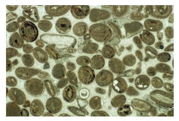
Sample: 8 SF: 908 Item: architrave Width of View of Picture: 3.4 mm Petrographic type: bioclastic oolitic grainstone with drusy spar cement Grain overcompaction: none Distinguishable bioclasts: echinoderm; probable calcite-replaced molluscs (upper left centre); probable oyster forming oolith nucleus at lower right corner.
