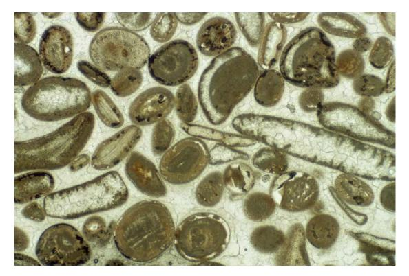
Sample: 13 SF: 835 Item: roughed-out mullion Width of View of Picture: 3.4 mm Petrographic type: bioclastic oolitic grainstone with drusy spar cement Grain overcompaction: none Distinguishable bioclasts: 2 large replaced probable mollusc fragments with well-developed micrite envelopes. Smaller central elongate grain may be punctuate terebratulid brachiopod.
