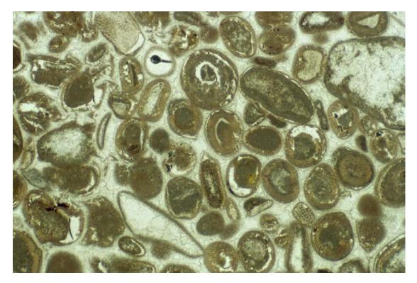
Sample: 10 SF: 858 Item: large moulding Width of View of Picture: 3.4 mm Petrographic type: bioclastic oolitic grainstone with drusy spar cement Grain overcompaction: none Areas of white space in some of the oolith cortices are due to fracture of the grains during the section-making process. Distinguishable bioclasts: echinoderm; calcite replaced probable aragonite molluscs
