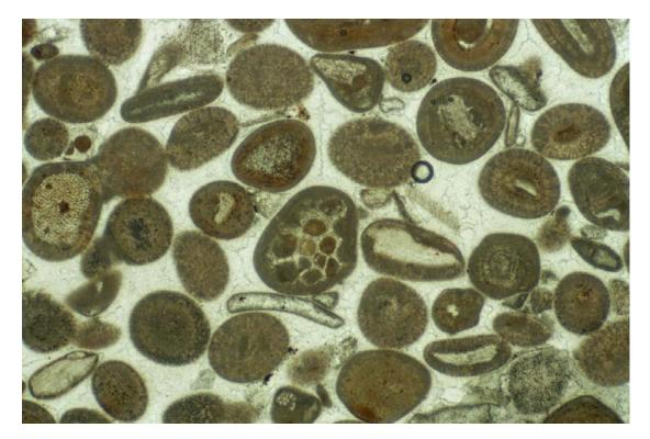
Sample: 19 SF: none Item: from core, 100 mm below hardground at top of Coombe Down Oolite Width of View of Picture: 3.4 mm Petrographic type: bioclastic oolitic grainstone with drusy spar cement Grain overcompaction: none
