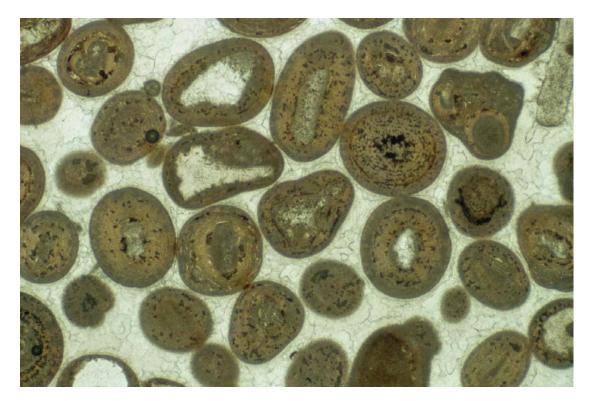
Sample: 6 SF: 945 Item: lip of sink Width of View of Picture: 3.4 mm Petrographic type: bioclastic oolitic grainstone with drusy spar cement Grain overcompaction: none Distinguishable bioclasts: calcite-replaced oolith nuclei, probably originally aragonite molluses.
