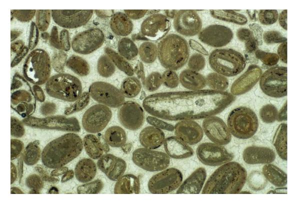
Sample: 5 SF: 881 Item: window moulding with glass groove Width of View of Picture: 3.4 mm Petrographic type: oolitic grainstone with drusy spar cement Grain overcompaction: none Distinguishable bioclasts: micromorphic gastropod; miscellaneous calcite-replaced molluscs.
