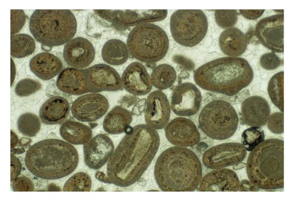
Sample: 15 SF: 139 Item: not identified Width of View of Picture: 3.4 mm Petrographic type: bioclastic oolitic grainstone with drusy spar cement Grain overcompaction: none Distinguishable bioclasts: none.
