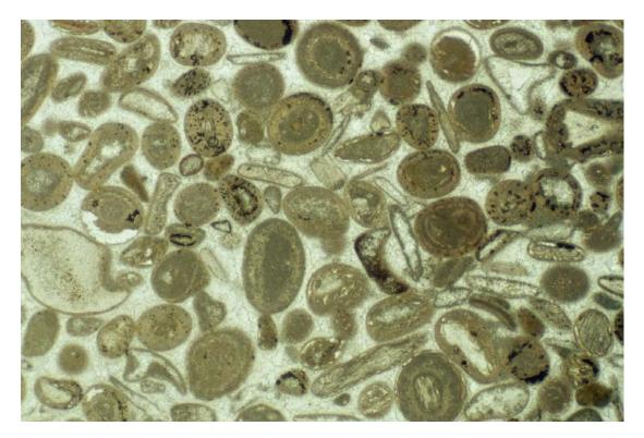
Sample: 2 SF: 398 Item: ridge stone tile Width of View of Picture: 3.4 mm Petrographic type: bioclastic oolitic grainstone with drusy spar cement Grain overcompaction: none Distinguishable bioclasts: echinoderm; miscellaneous calcite-replaced molluscs; probable oyster.
