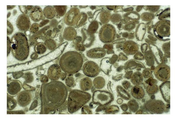
Sample: 14 SF: 670 Item: block for crane bottom Width of View of Picture: 3.4 mm Petrographic type: bioclastic oolitic grainstone with drusy spar cement. Traces of micrite locally between grains Grain overcompaction: none Distinguishable bioclasts: calcite-replaced probable mollusc fragments.
