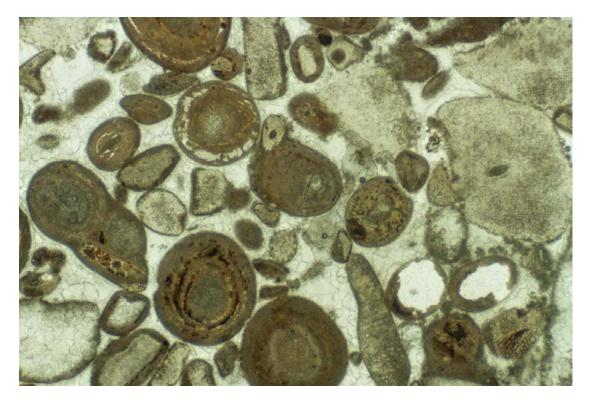
Sample: 12 SF: 731 Item: large block from behind roof fall; Ralph Allen's time Width of View of Picture: 3.4 mm Petrographic type: oolitic bioclastic grainstone with drusy spar cement and prominent echinoderm debris Grain overcompaction: none Areas of white space in some of the oolith cortices are due to fracture of the grains during the section-making process.
