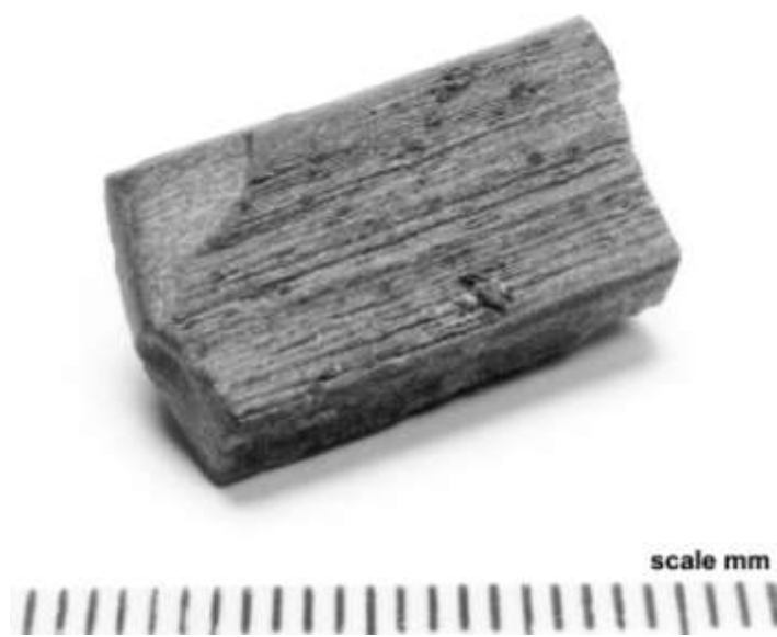
Figure 1. The strip of red glass showing the surface striations (scale is in mm)
