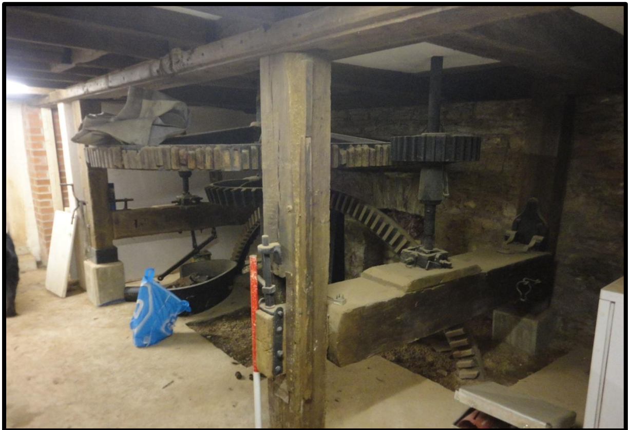
Fig. 5 View of the mill machinery on the meal floor showing the pitwheel and spurwheel underdrives providing power to two sets of stones.
