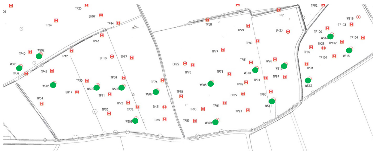
Figure 5 Detail of the central southern portion of Figure 1 to show the location of the various Window Samples (highlighted in green). Not to scale.
