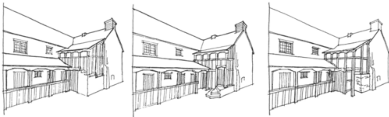
Figure 11.25 (above) Design proposals for the reinstatement of first-floor access via a partially reinstated gallery; key points are the roof pitches and the relationship between pentice and gallery, which was lost in the completed work (see Fig 11.24) where the open bay of the pentice is too wide (drawings by Mark Samwell, c January 1994).
