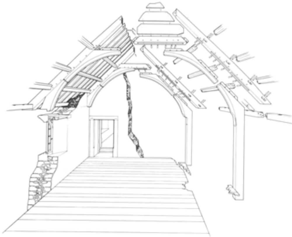
Figure 7.27 Exploded analytical drawing of the roof of the south range (inner chamber), looking west, with truss VII in the foreground (not to scale) (line drawing by Piran Bishop).
