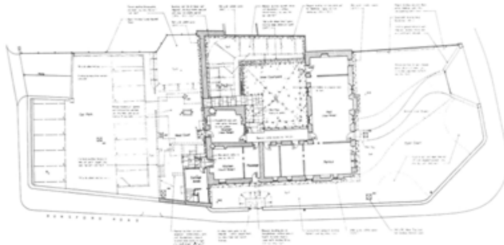
Figure 11.6 Layout of the site and ground-floor plan of the house at the penultimate stage to completion, before the east car park was added. The west car park, with its double row of parking spaces, encroaches more on the building than the car park in Slade's original proposal (Fig 11.3). With the addition of the later eastern car park the building is surrounded. The main public entrance is now via the west service room from the west car park. The stairs in the south-west annexe are now the only means of access to the first floor. Note the lines of the missing north and west sections of the building set out in the inner courtyard (not to scale) (April 1994; AL/SK/03/A).
