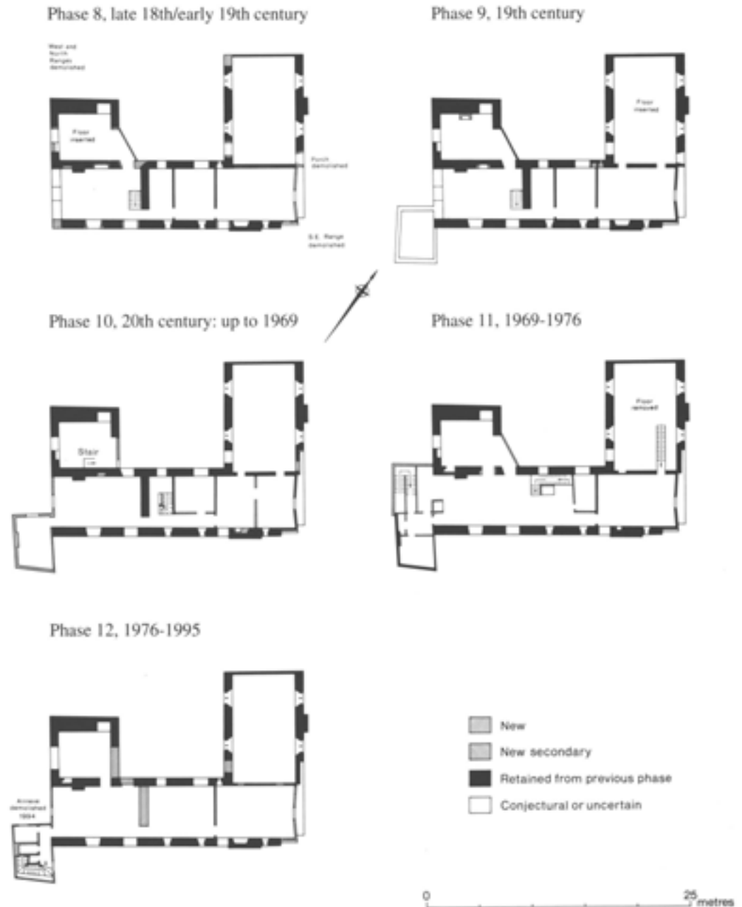
Figure 12.4 Phased plans to illustrate the development of the site: first floor, phases 8–12 (scale 1:500) (line drawing by Tony Ives).
