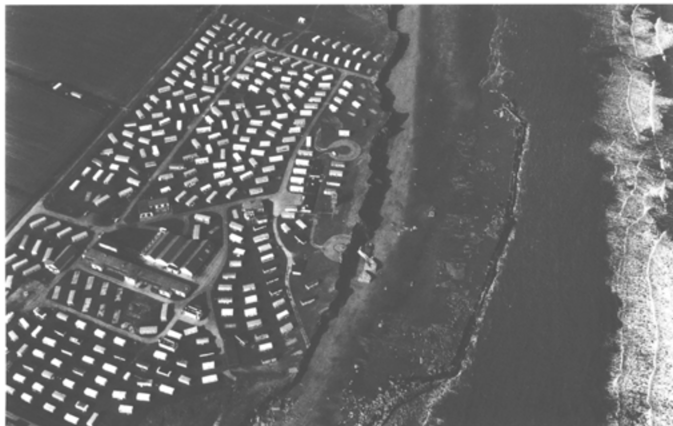
Fig 41 Kūnsea, Humberside, three miles north of Spurn Head on the North Sea coast. The photograph illustrates dramatically the effect of coastal erosion both on the modern caravan park and on the circular WW II gun platforms, one of which has already been cut in half (centre/middle). NMR 12364/49. (RCHME © Crown copyright)
