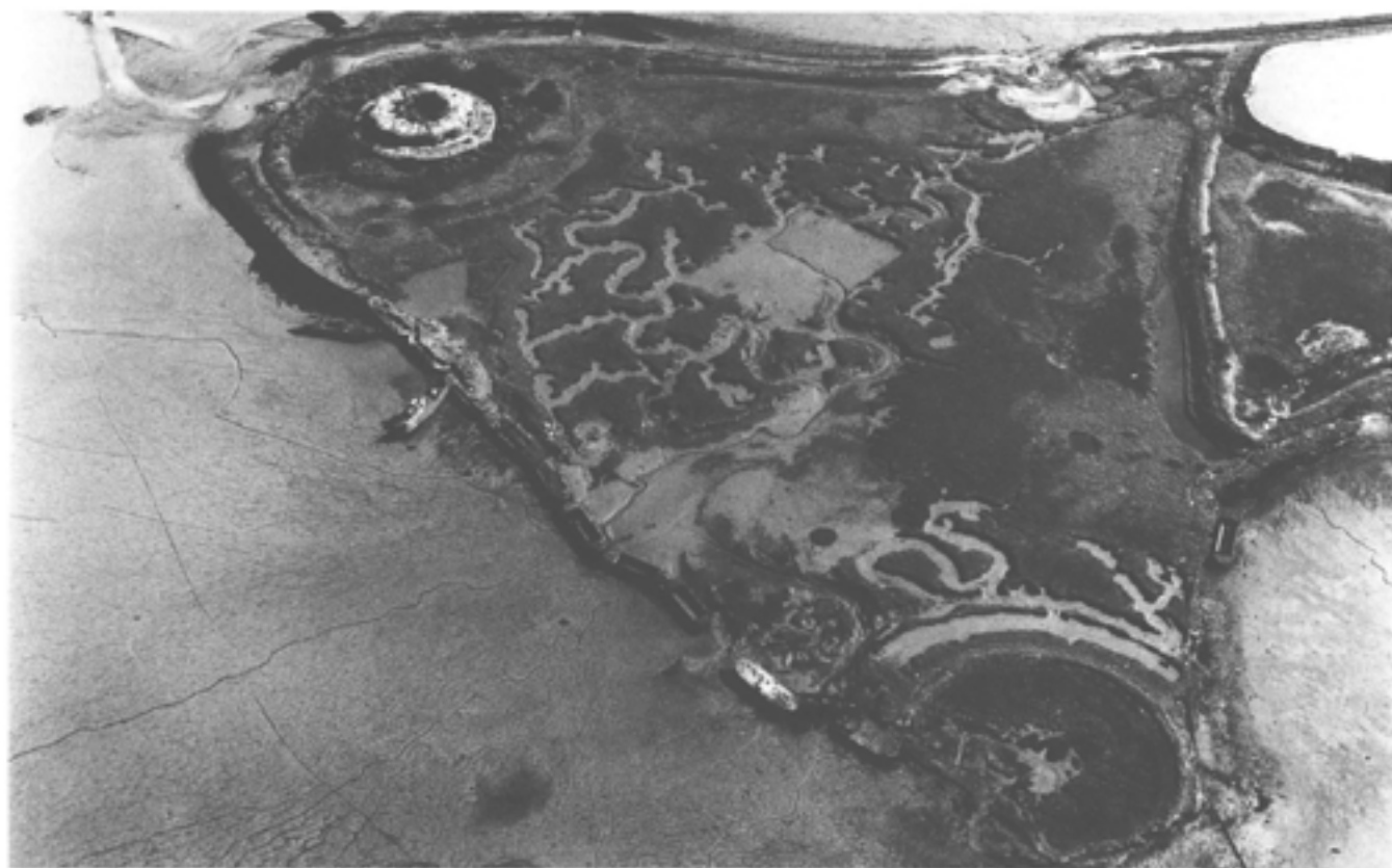
Fig 42 Hoo Fort on the river Medway, Kent, with sea defences constructed from barge hulks. TQ 7970/16 (RCHME © Crown copyright)
