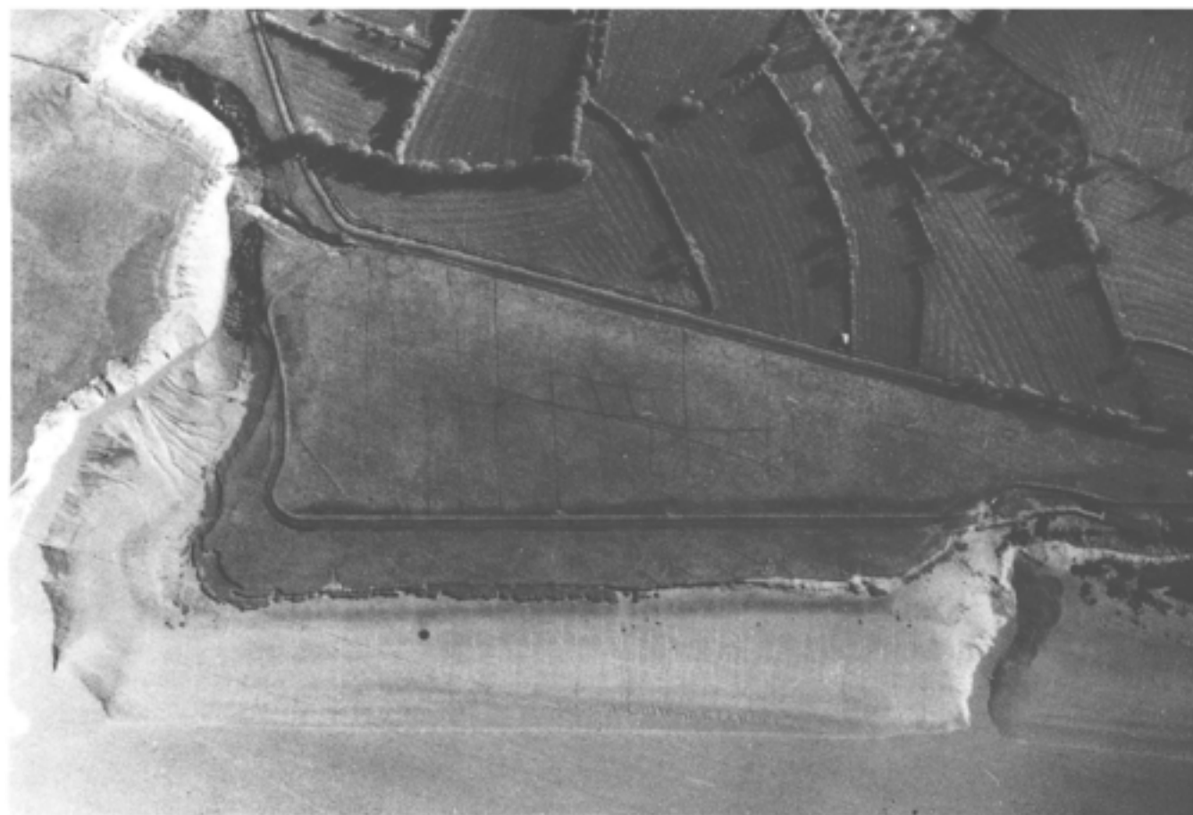
Fig 72 Cowhill Warth on the south bank of Oldbury Pill, Gloucestershire (area approximately 600 x 400m). The main sea-bank has been set back across the ridge-and-furrow contained in the hedged fields
