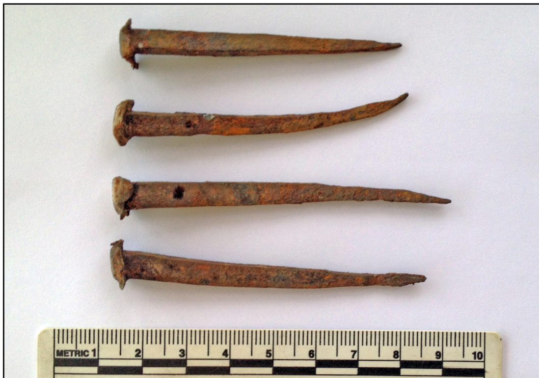
Appendix I.20: Detail of hand-made iron nails (10cm scale).
