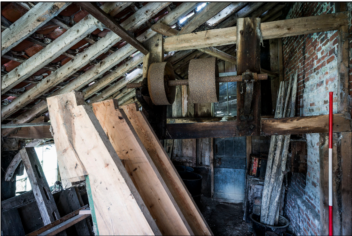
Appendix 2.70: Detail of overhead belt wheels for power drive to former saw bench in room 3G5 (2m scale). Photo No.44
