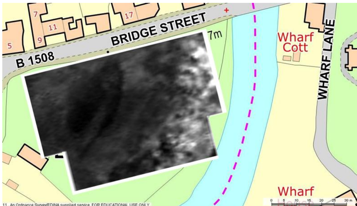
Figure 6: Geophysical survey of Bures Common carried out in summer 2012 in advance of the 2012 excavations. Areas of higher resistance are light in colour, areas of low resistance are show darker.
