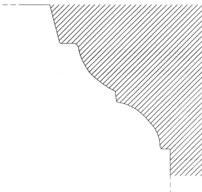
Moulding Profile of Ceiling Cornice on North and South Walls of Ground Floor South Room
