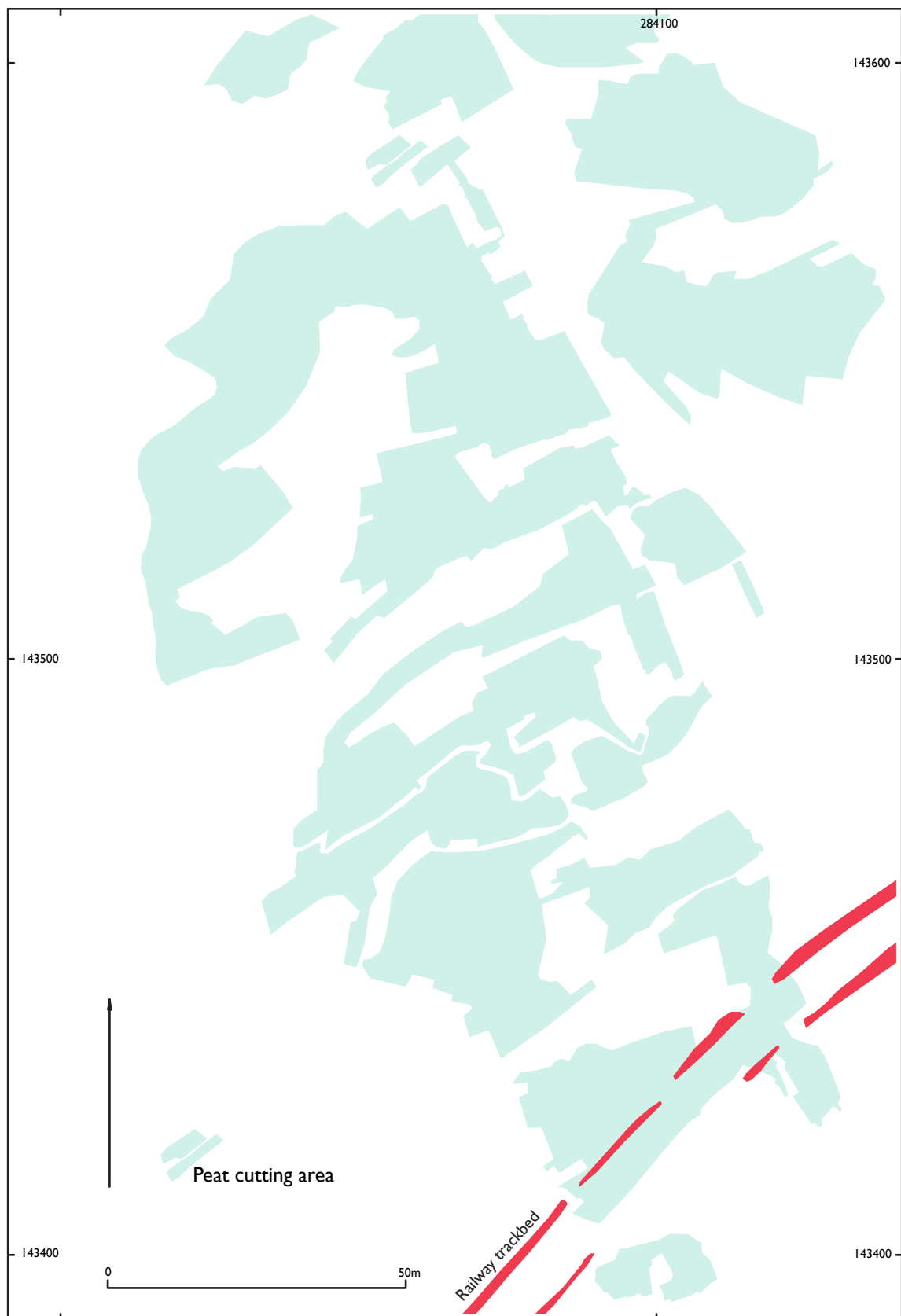
Fig 67 Survey of the Simonsbath-Porlock railway trackbed built across disused turf pits (1:1000)
