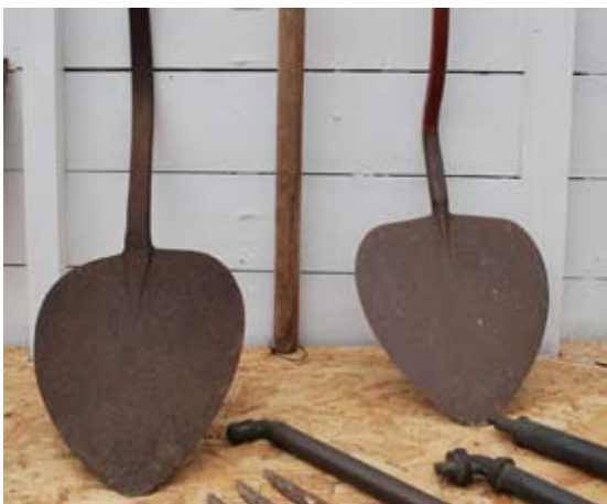
Fig 22 (below) Detail of the heart shaped blades of the turf cutting spades in the West Somerset Rural Life Museum (Hazel Riley)
