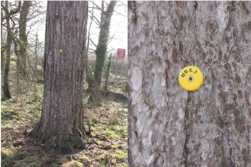
*Figure 4.3 Tree control points. Locations established in relation to TBMs using Total Station. These and the TBMS were then used to situate the Semi-Permanent control points established around the pit.*
