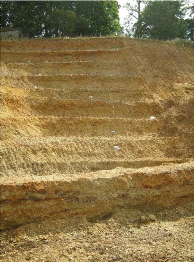
Figure 5.4 The stepped face of Hodge Ditch I used for cosmogenic sampling. Note the bags at sample locations and the OSL holes at the base (CHAR 22 and CHAR 21).
