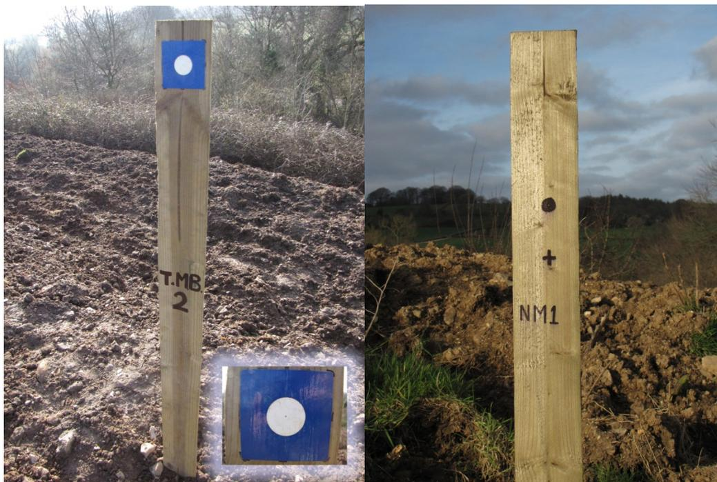
Figure 4.6 Semi-permanent Control Targets on posts. Example on the left is the Leica stickers, and on the right is the marker pen trial version
