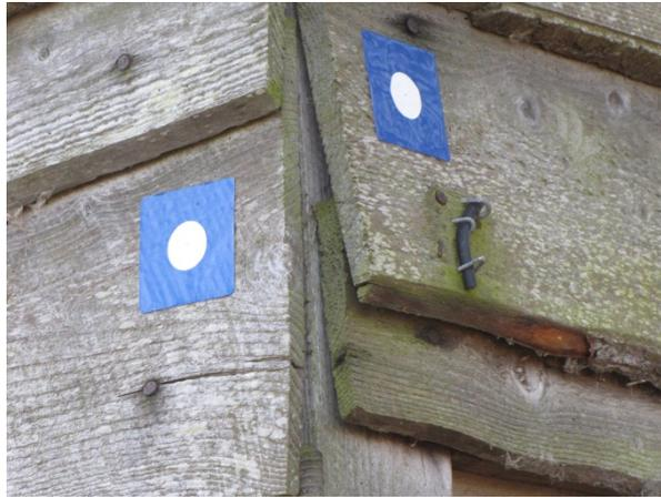
Figure 4.5 Control Targets on shed in HD1
