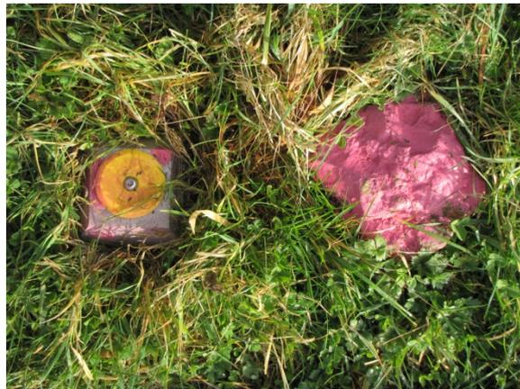
*Figure 4.1 Example of metal Temporary Bench Mark in ground surveyed in using differential GPS*
