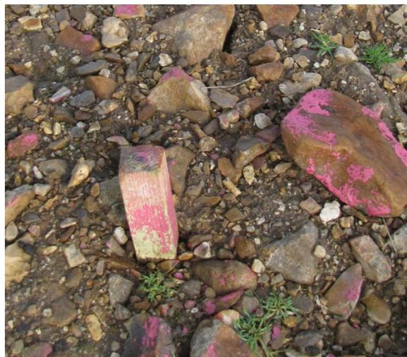
*Figure 4.2 Example of wooden post used as Temporary Bench Mark in areas likely to be excavated or landscaped resulting in the destruction of the point. These were surveyed in using differential GPS.*
