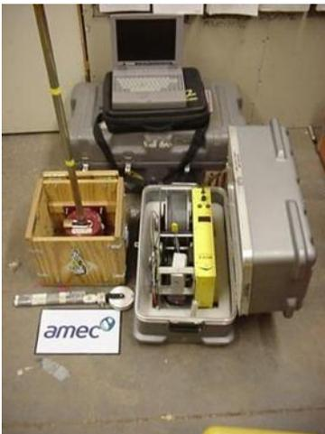
Figure 2.1 Commercial gamma cps equipment rig. Picture courtesy of Amec Ltd..
