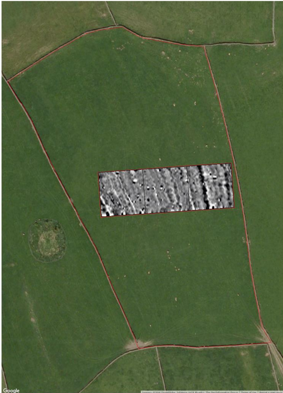
Figure 5: Site 1, Magnetic Survey over Google Satellite image (Range -3nT to +3nT)
