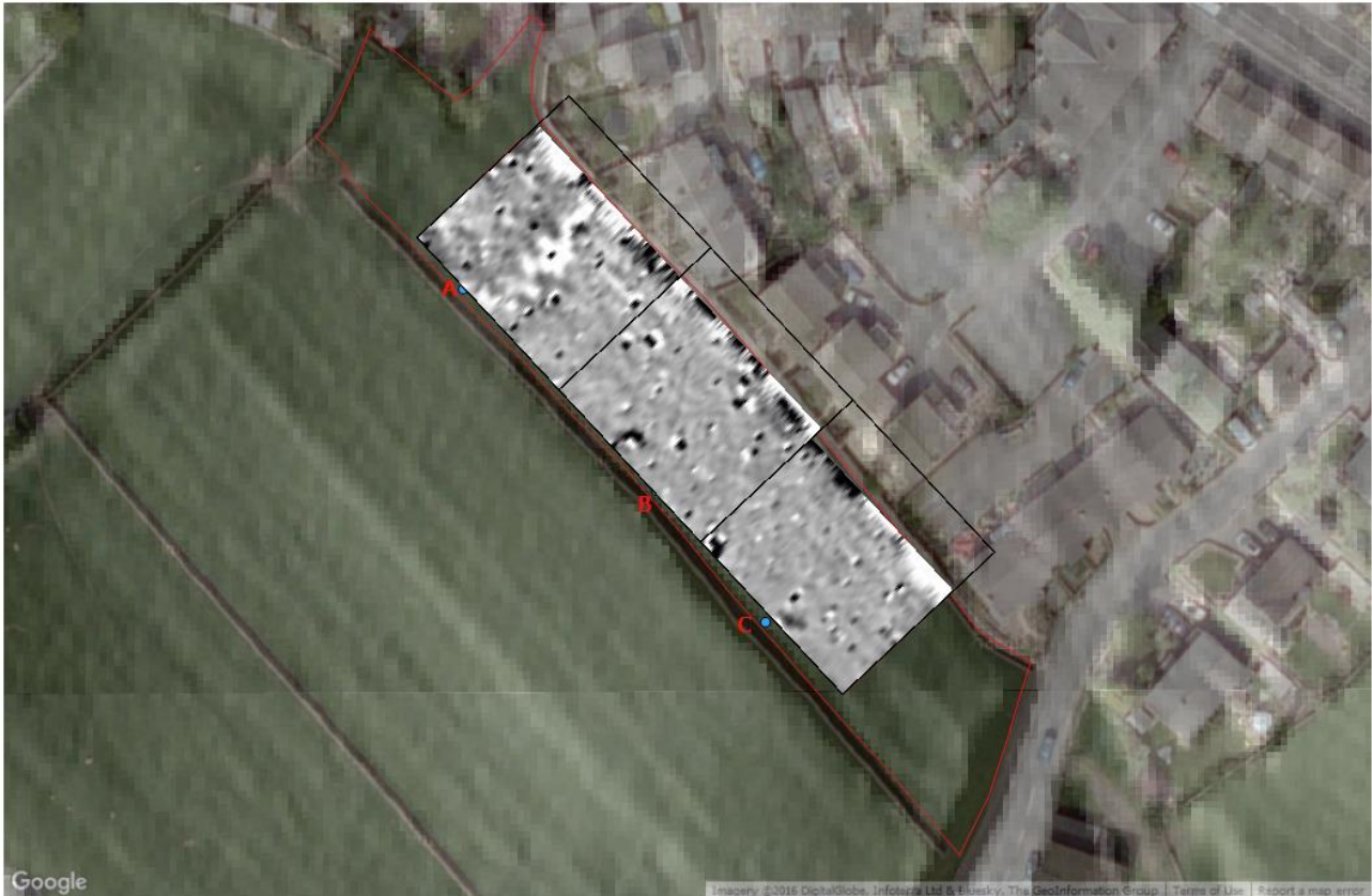
Figure 12: Site 2, Magnetic Survey data superimposed over LIDAR at 50% transparency over Google Earth image. (Range -5nT to +10nT)
