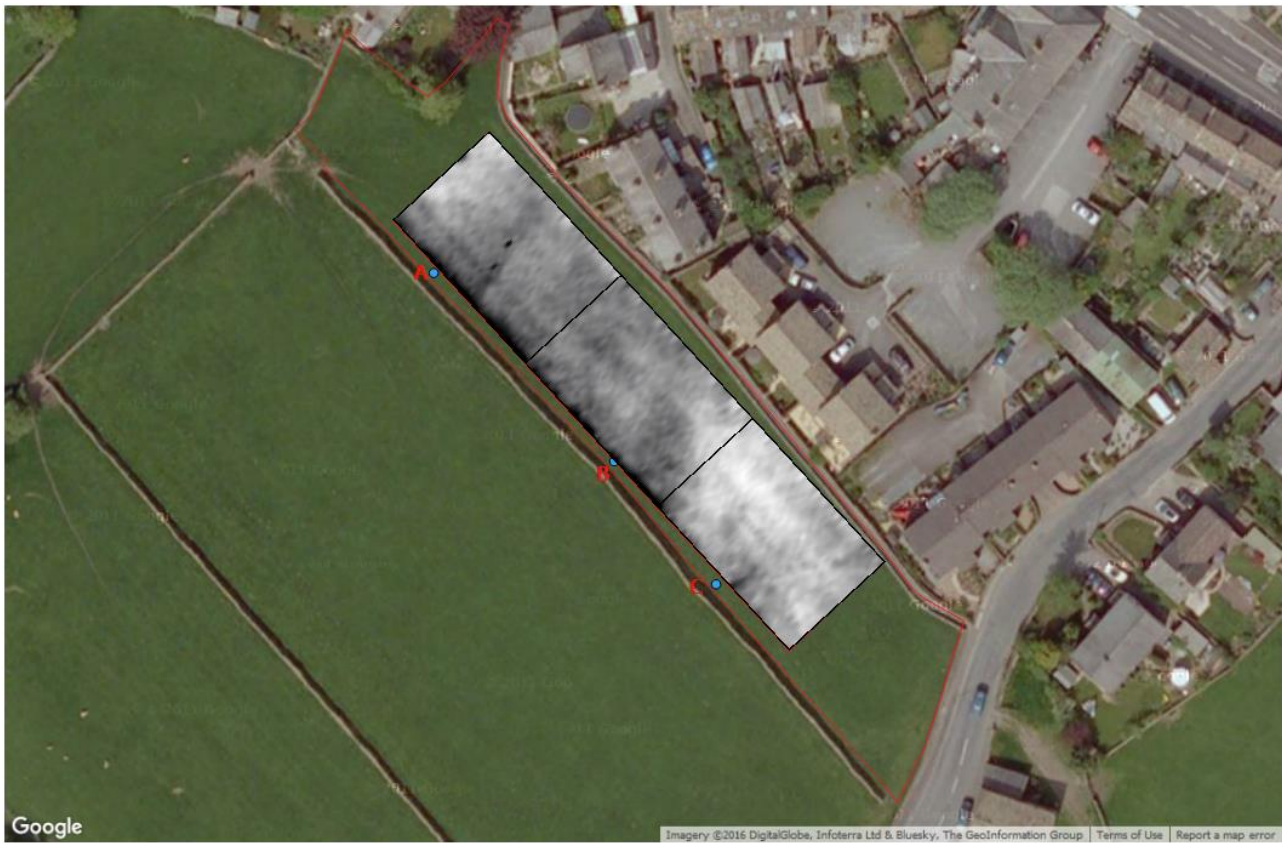
Figure 14: Site 2, Processed Resistance Survey data superimposed over Google Satellite image. (Clipped at \pm 2SD )
