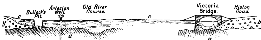
Fig. 9. Diagram Section from Park Street to Victoria Bridge. a. Gault. b. Gravel. c. Alluvium.
