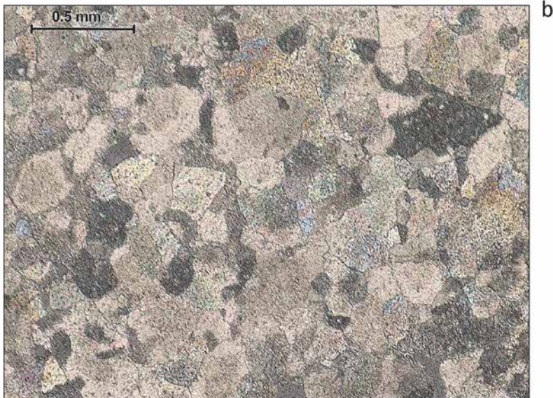
Figure 46 a-b: Photomicrographs coarse Magnesian Limestone both from Arbeia, sourced from the Cleadon Hills. Used in small amounts at St. Paul's, Jarrow in the pre-Conquest and later phases. Also used occasionally in the pre-Conquest fabric at St. Peter's, Wearmouth.
