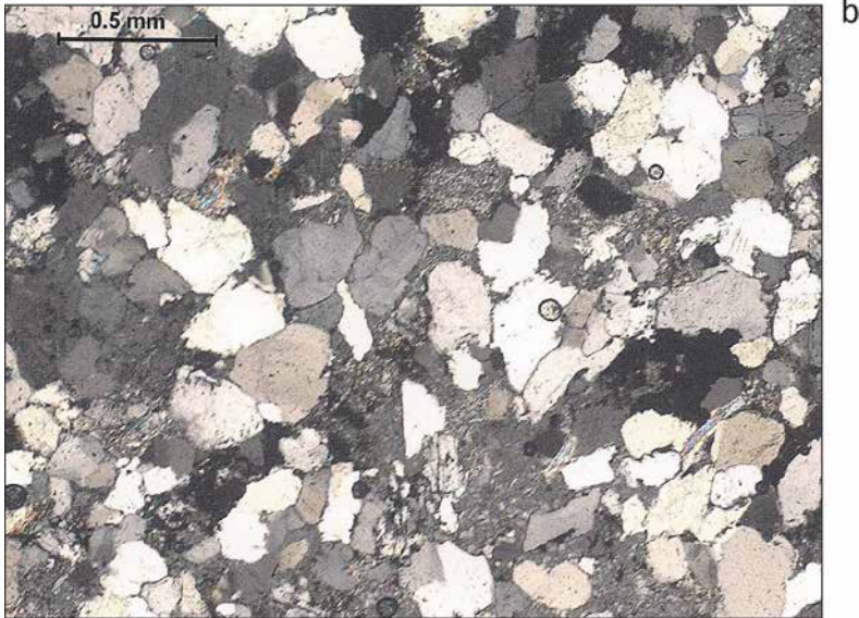
Figure 50 a-b: Sandstones a) photomicrograph burrows in Type F sandstone from St Paul's, Jarrow (polarised light) b) Type H (Heworth) Sandstone (polarised light), St. Paul's, Jarrow.
