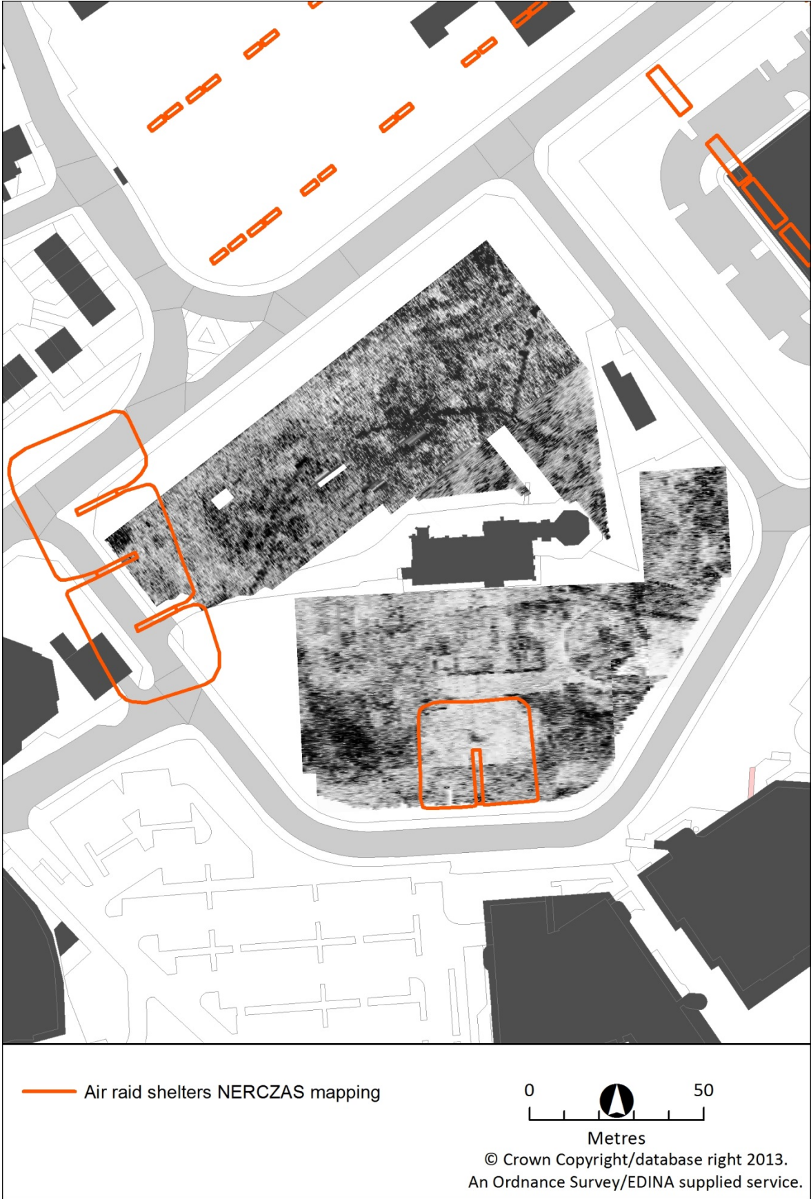
Figure 136: NERCZAS mapping of WWII air raid shelters and GPR plot c.1.0 metres
