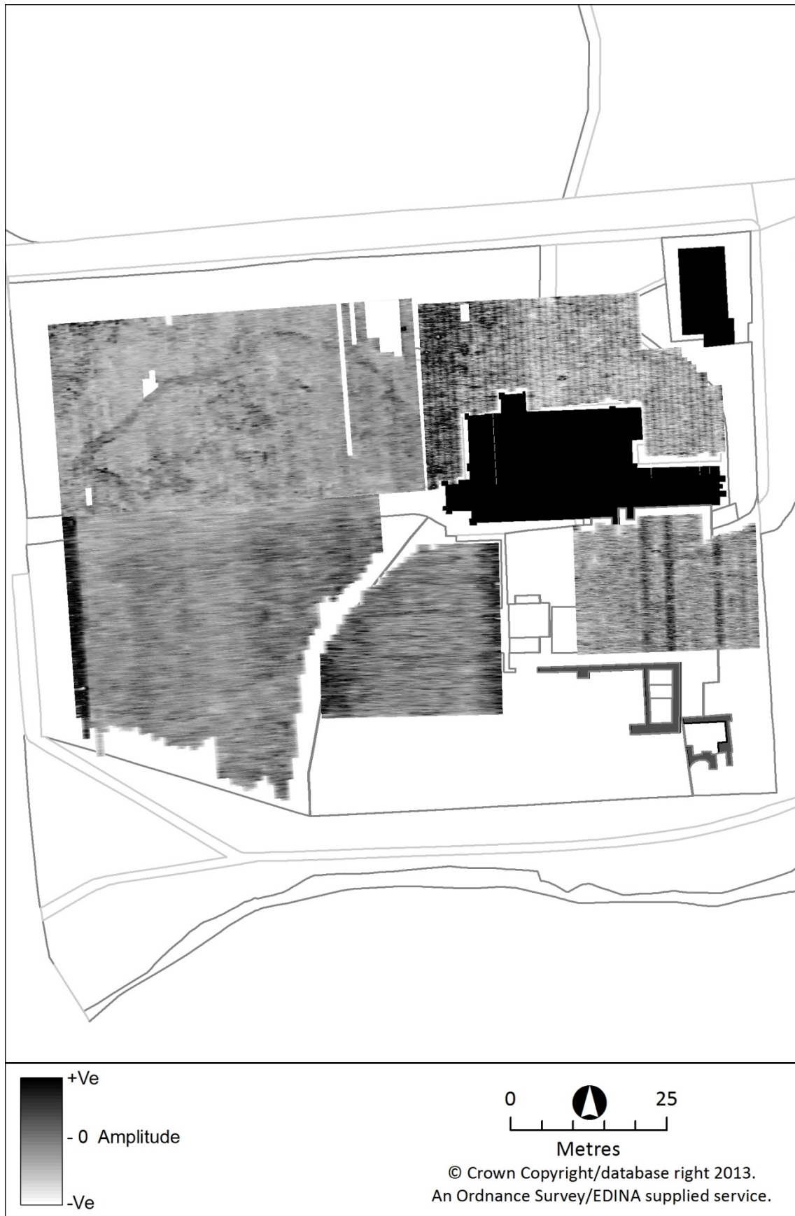
Figure 73: GPR survey results, St Paul's Church, Jarrow, 2009 – depth c.275cm
