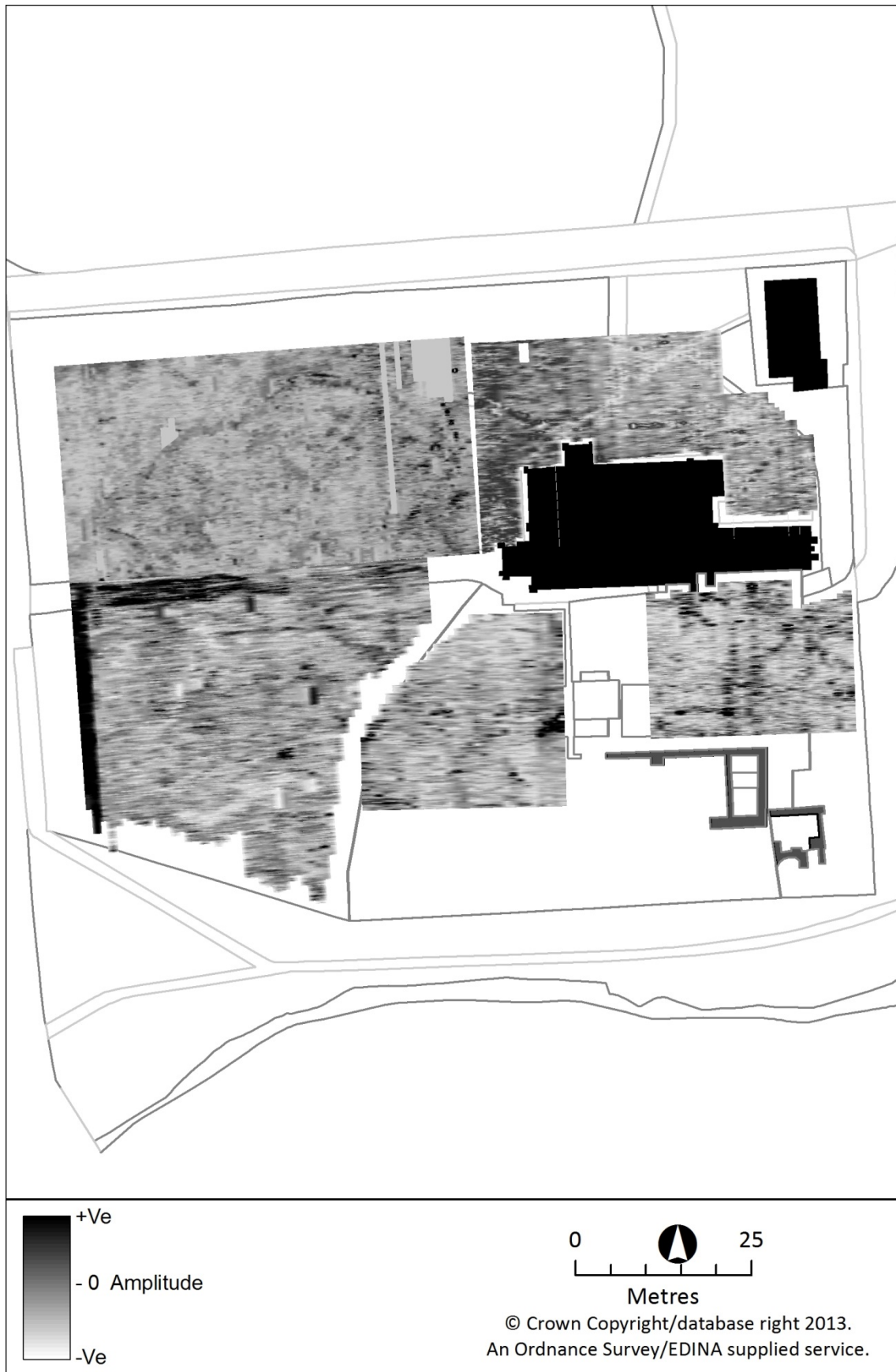
Figure 66: GPR survey results, St Paul's Church, Jarrow, 2009 – depth c.75cm
