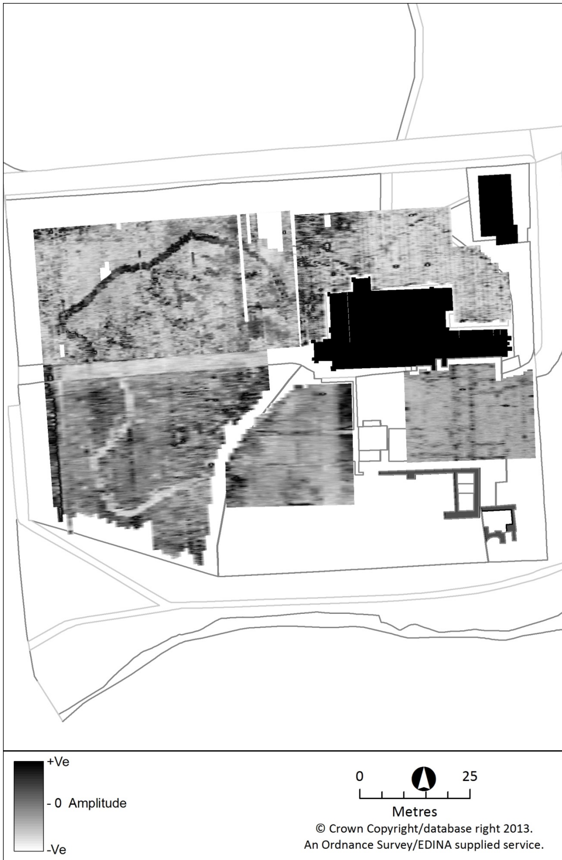
Figure 70: GPR survey results, St Paul's Church, Jarrow, 2009 – depth c.175cm
