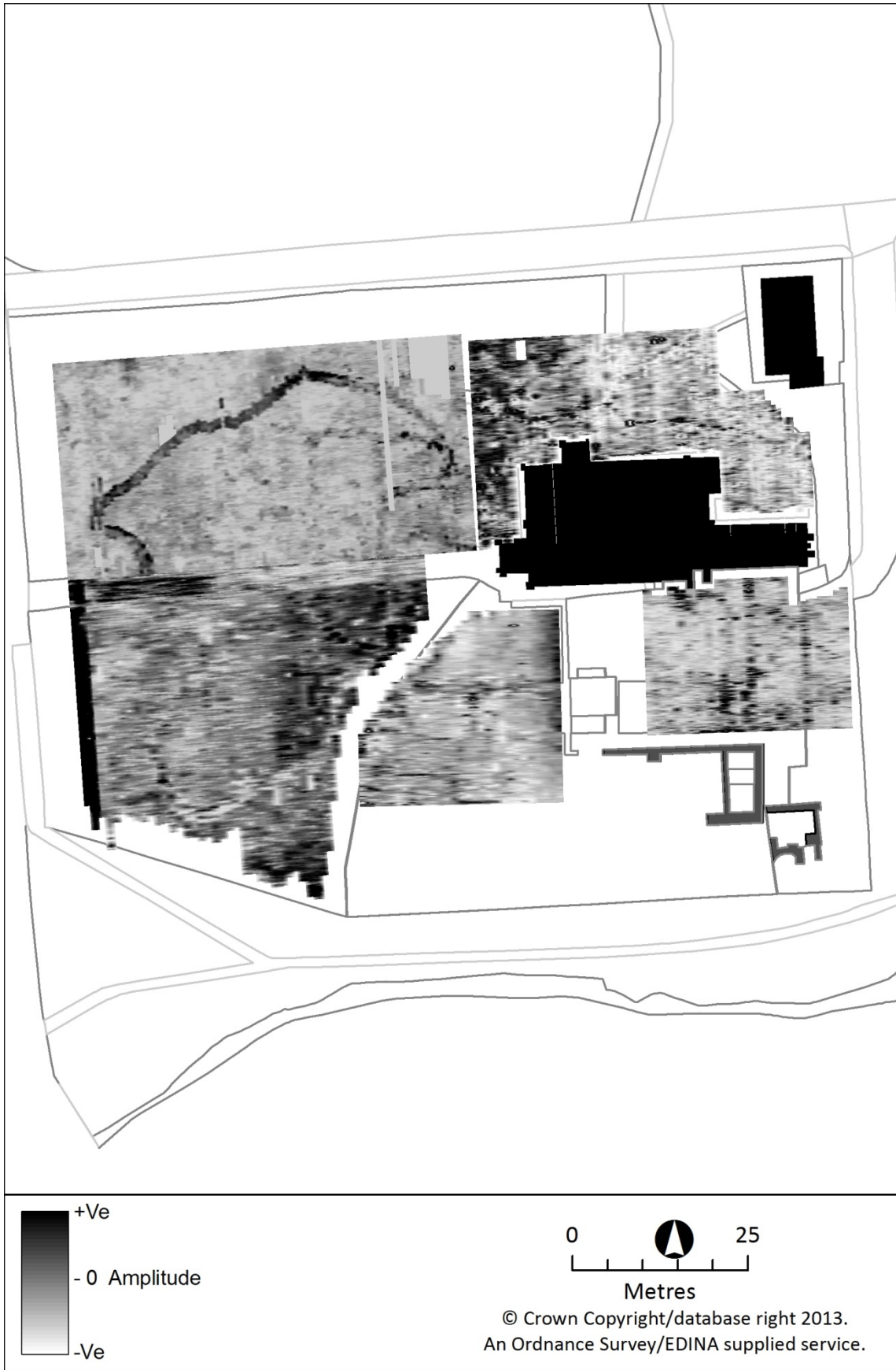
Figure 67: GPR survey results, St Paul's Church, Jarrow, 2009 – depth c.100cm
