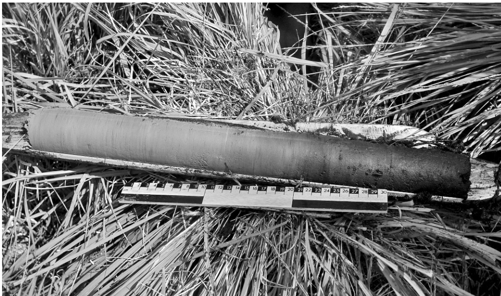
FIG 2. Transition from peats to clay laid down in open water. Core from 50 – 100cm. The upper section of the core is to the right and shows dark peats which slowly change into the lighter coloured clays. The material for radiocarbon dating came from 60-61.5cm.
