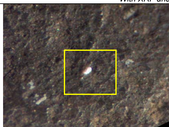
Figure 3: Touchstone D2180 Detail of the surface under binocular microscope, with SEM analysis localisation (Area 1)
