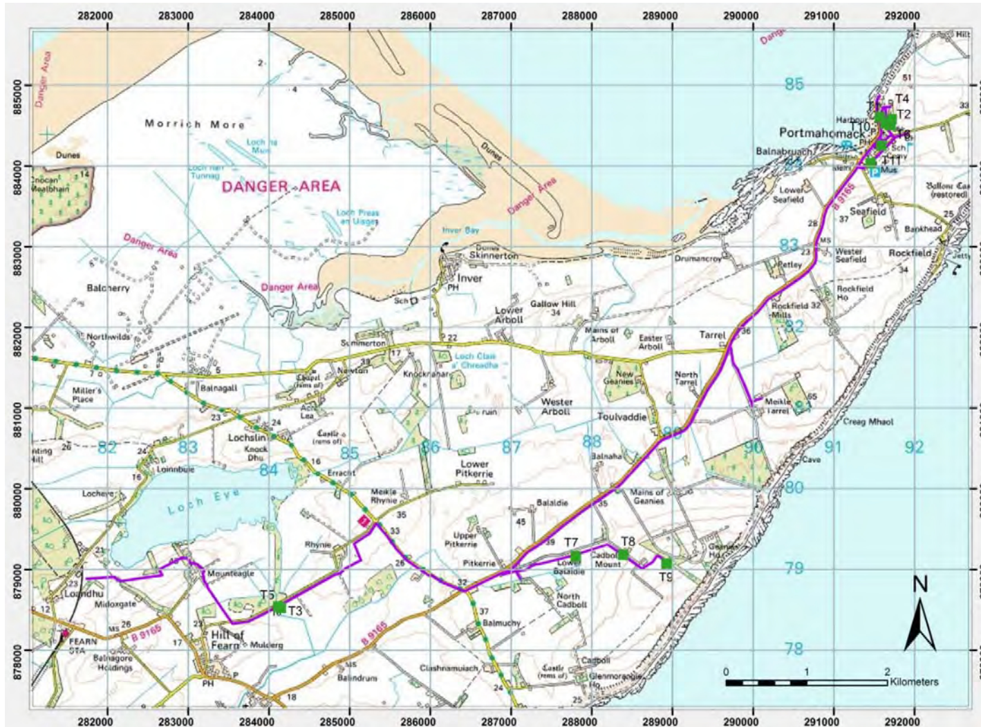
Figure 2 Water main line and WB trenches
