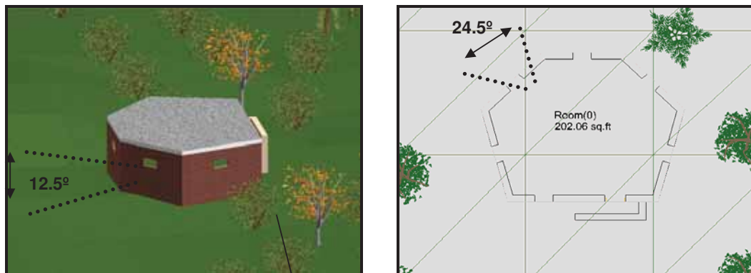
Fig.46 – FW3 / 24SP pillbox displaying visibility angles afforded by the loopholes 1 (© IMSI TurboCAD Deluxe v9)
