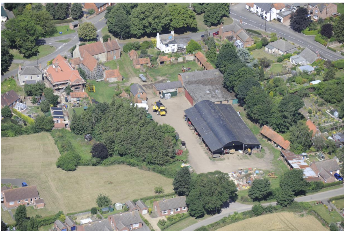
Manor Farm, Helpringham. A regular 'U' plan farmstead with a large detached farmhouse. Note the modern farm building in the foreground for the storage of arable crops. The cattle sheds and crew yard are now disused
