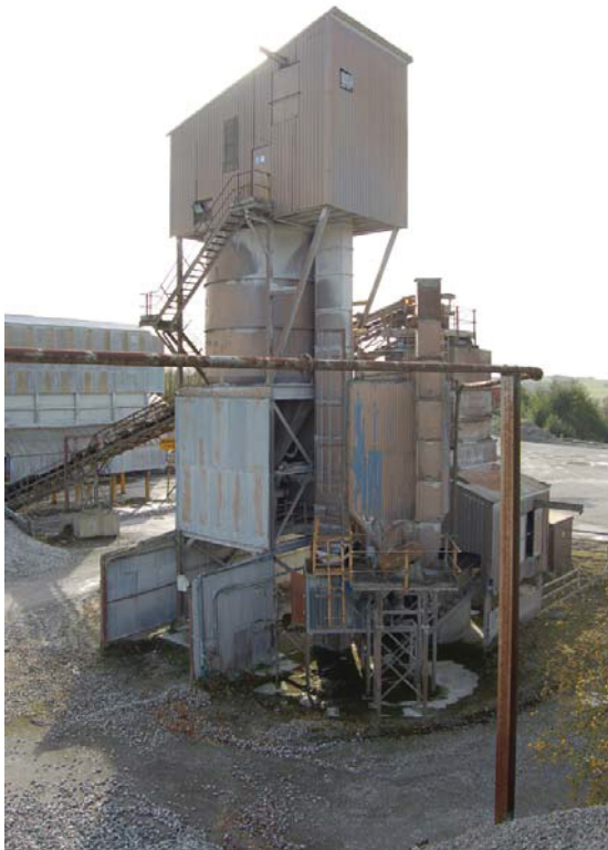
Plate 27: 'Stock A Coating Plant' [21], NT SMR 54,220 . View from north; note bucket elevator and dust extractor.
