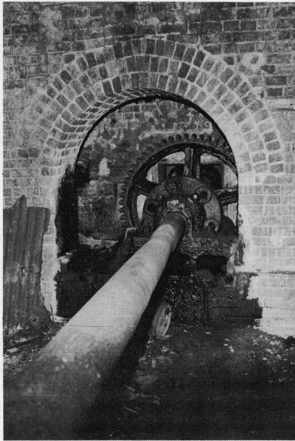
Plate 21 The line-shaft passing through the opening between Chambers C and D (see Fig. 19)
