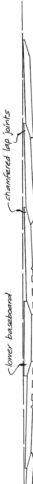
Section through Boards at A - A
