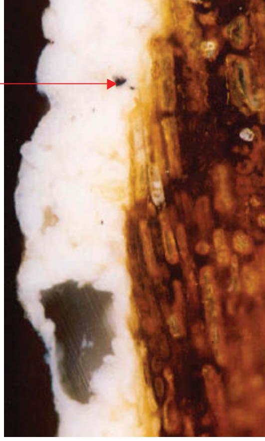
Sample 18 photographed in cross-section under reflected light at 200x magnification. (Printed magnification not calculated).
