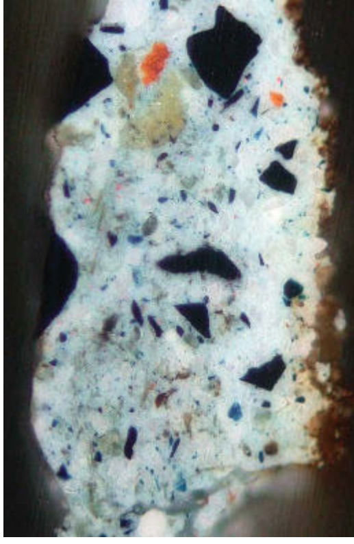
Sample 1 (3070) photographed in cross-section under reflected light at 200 x magnification. (Printed magnification not calculated).
