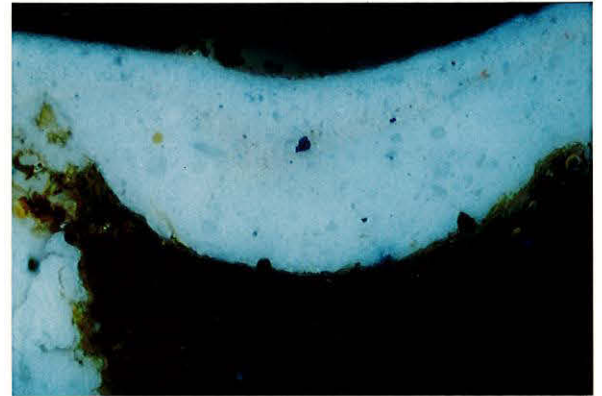
Plates 58 ( below ). Detail of wave-pattern border surrounding St. Peter. Plate 59 ( above ). Cross-section of Sample 26/2118 at 1208 x magnification, showing the wood support over which a layer of lead white is evident. A trace of vermilion is apparent towards the upper part of this thick white layer which compares closely to that found in Sample 27. A thick accretion of surface dirt is visible at the top of the sample. ( Macrophotograph Heritage/Howard 1997, photomicrograph Howard 1997 ).
