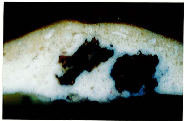
Plates 65 ( above ). Cross-section of Sample 29/2121 taken from a brown 'stain' on the extended chevron pattern border surrounding St. Peter, shown at 1200x magnification. The brown appearance of the surface is clearly due to a coating which has penetrated into the lead white paint layer. ( Photomicrograph Howard 1997 ).
